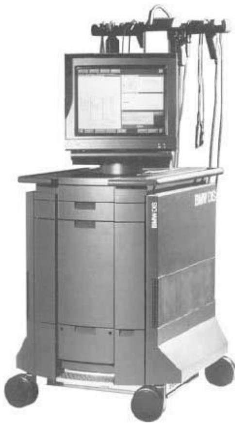
Fig. 4: Diagnosis And Information System (DIS) Tester Courtesy of BMW OF NORTH AMERICA, INC.
