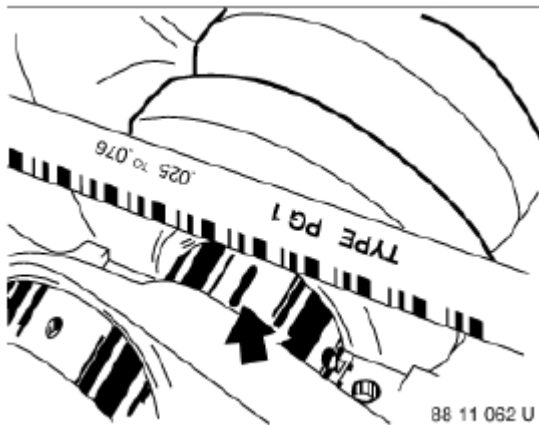
Fig. 142: Checking Main Bearing Play Courtesy of BMW OF NORTH AMERICA, INC.
