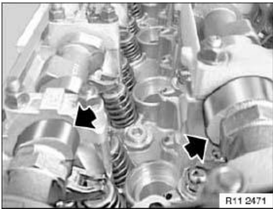
Fig. 444: Locating Crank Engine Central Bolt In Direction Of Rotation To Firing TDC Position Courtesy of BMW OF NORTH AMERICA, INC.
