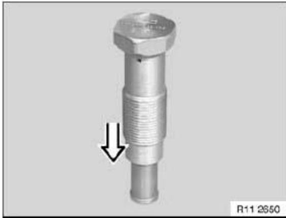
Fig. 77: Compressing Chain Tensioning Piston On Level Surface Courtesy of BMW OF NORTH AMERICA, INC.
