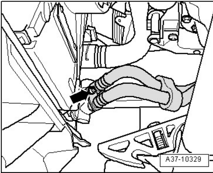
Fig. 53: Identifying Lines From Transmission Oil Cooler And Rear Mounting Bolts Courtesy of AUDI OF AMERICA, LLC
