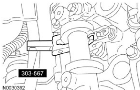
Fig. 127: Compressing Valve Spring Using Valve Spring Compressor Courtesy of FORD MOTOR CO.
