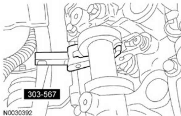
Fig. 345: Compressing Valve Spring Using Valve Spring Compressor Courtesy of FORD MOTOR CO.
