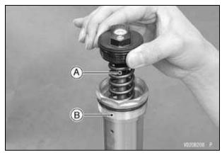
A. Left Front Fork Base Valve Assembly B. Left Front Fork Cylinder Unit
