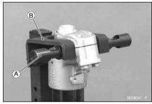
A. Holder Bar of Fork Spring Compressor (Special Tool: 57001-1587)
