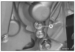
A. Coolant Drain Bolt
