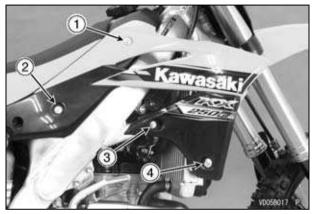
• Tighten the radiator shroud bolts securely.
