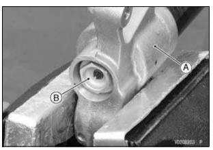
A. Axle Holder Part B. Left Front Fork Adjuster Assembly
