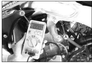
A. Idle Adjusting Screw/Choke Knob B. Tester
