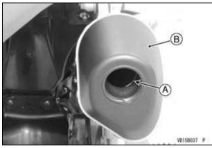
A. Muffler Pipe End B. Baffle
