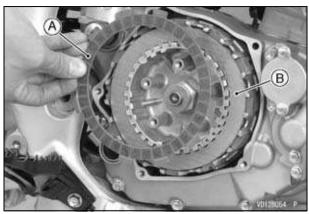
A. Friction Plate B. Steel Plate
