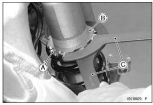
A. Spring Preload Adjusting Nut
