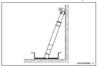
Holding the top plug wrench (special tool: 57001 -1645) with a vise, loosen the left front fork base valve assembly on the fork cylinder unit with a box wrench.
