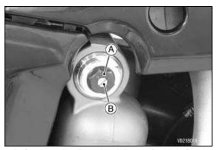
A. Compression Damping Adjuster for High Speed B. Compression Damping Adjuster for Low Speed
