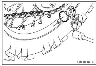
A. Axial Rim Runout Measurement
