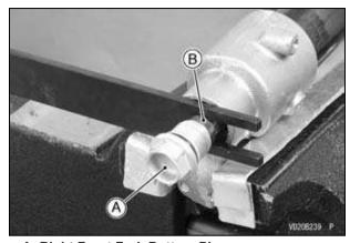
A. Right Front Fork Bottom Plug B. Right Front Fork Bottom Plug Locknut
