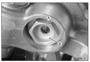
A. Rebound Damping Adjuster B. Left Front Fork Cylinder Valve
