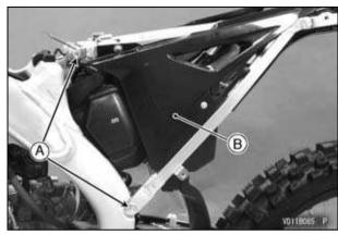
A. Rear Frame Mounting Bolts B. Air Cleaner Housing
