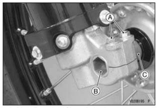
A. Right Front Axle Clamp Bolts (Loosen)
