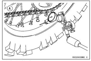
A. Radial Rim Runout Measurement
