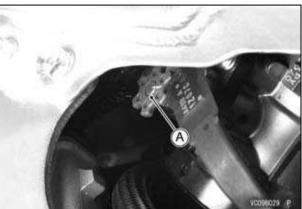
A. Idle Adjusting Screw/Choke Knob
