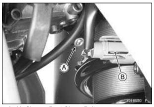
A. Air Cleaner Duct Clamp Bolt B. Intake Air Temperature Sensor Connector
