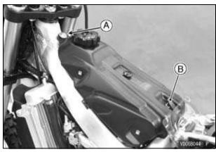
A. Fuel Tank Mounting Bolt B. Band
