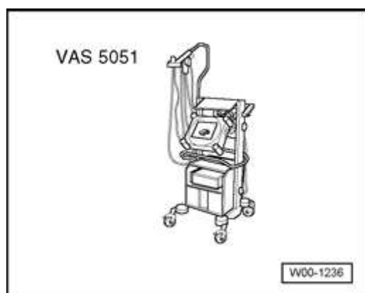
Fig. 19: VAS 5051 Vehicle Diagnosis, Testing and Information System Courtesy of VOLKSWAGEN UNITED STATES, INC.
