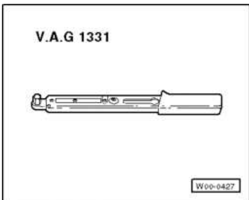
Fig. 54: Torque Wrench V.A.G 1331 Courtesy of VOLKSWAGEN UNITED STATES, INC.
