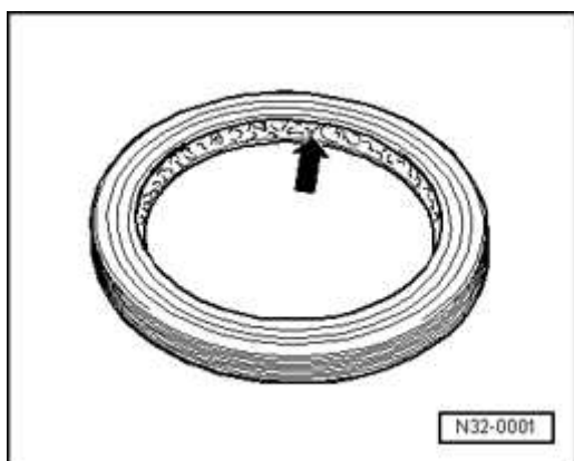
Fig. 4: Identifying Space Between Oil Seal Sealing Lips Courtesy of VOLKSWAGEN UNITED STATES, INC.
