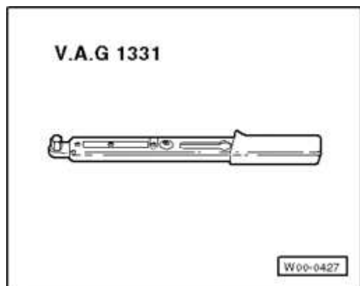
Fig. 48: Torque Wrench V.A.G 1331 Courtesy of VOLKSWAGEN UNITED STATES, INC.
