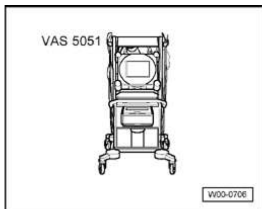
Fig. 22: VAS 5051 Vehicle Diagnosis, Testing & Information System Courtesy of VOLKSWAGEN UNITED STATES, INC.
