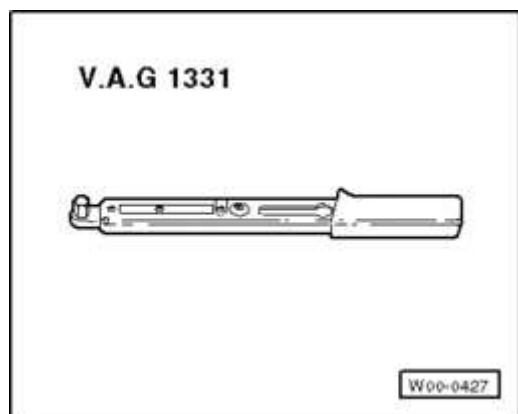
Fig. 118: Torque Wrench V.A.G 1331 Courtesy of VOLKSWAGEN UNITED STATES, INC.
