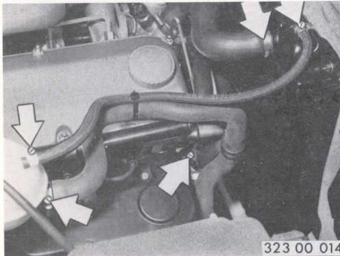
Take up slack at all hose clips on radiator and coolant expansion tank.
