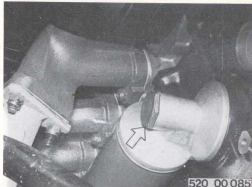
*When installing:* Place adaptor in lock. Renew aluminum seal. Tightening torque:<sup>1)</sup>
