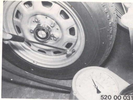
**17. Checking/adjusting toe of front wheels**
