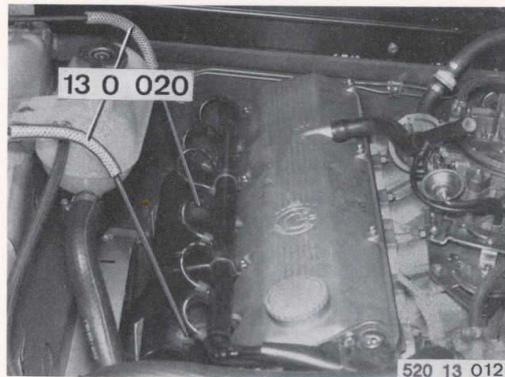
Adjust CO level with the mixture control screws (2 and 3).<sup>1)</sup>
