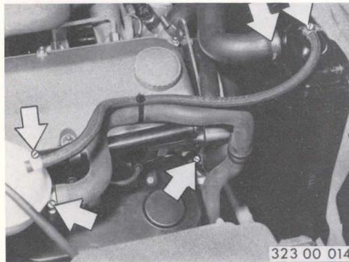
**Tighten all hose clips on radiator and expansion tank.**
