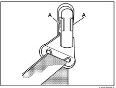
To move it up or down, squeeze the release buttons (A) together and move the height adjuster to the desired position.
