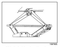
With the jack head positioned correctly on the metal jacking flange, it should look like this from underneath.
