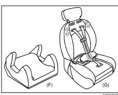
A booster seat (F-G) is a child restraint designed to improve the fit of the vehicle's safety belt system. Some booster seats have a shoulder belt positioner, and some high-back booster seats have a five-point harness. A booster seat can also help a child to see out the window.
