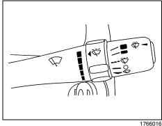
Use the lever on the right side of the steering column to operate the windshield wipers.
