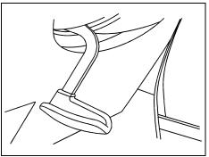
The lever to tilt the steering wheel is located on the left side of the steering column.
