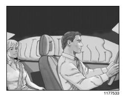
The roof-mounted rollover airbag for the driver and the person seated directly behind the driver is located in the ceiling above the side windows.
