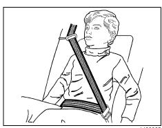
4) Buckle, position, and release the safety belt as described in "Rear Seat Passengers" in this section. Make sure that the shoulder belt crosses the shoulder.
