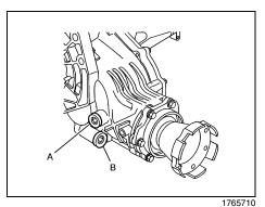
A. Fill Plug B. Drain Plug To get an accurate reading, the vehicle should be on a level surface.
