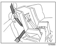
6) To tighten the belt, push down on the child restraint, pull the shoulder portion of the belt to tighten the lap portion of
