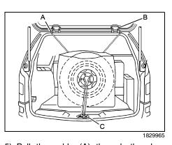
5) Pull the cable (A) through the door striker (C) and the center of the wheel.
