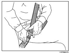
To unlatch the belt, push the button on the buckle. The belt should go back out of the
