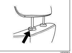
Pull the head restraint up to raise it. To lower the head restraint, press the button, located on the top of the seatback, and push the restraint down.
