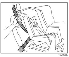
5) To tighten the belt, push down on the child restraint, pull the shoulder portion of the belt to tighten the lap portion of
