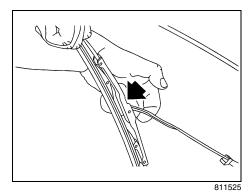
3) Pull up the release clip, located at the connecting point of the blade and the
