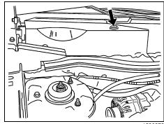
1) Remove the push pins from the rear of the passenger's side air inlet panel. It is located in the rear of the engine com-
