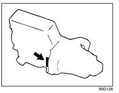
The engine serial number is stamped on the cylinder block as shown in the above illustration.
