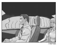
The roof-mounted rollover airbag for the right front passenger and the person directly behind that passenger is located in the ceiling above the side windows.
