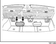
The third row seat head rests can be removed from the seatback. To do this, press the button, located on the top of the seatback, and pull them out from the seatback. Store the head rest, front side facing up, in the compartment behind the third row, by inserting the head rest posts into the slots in the storage area.
