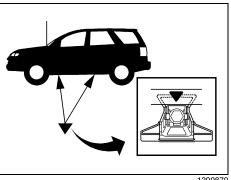
4) Find the arrow on the plastic lower body panel. Position the jack head under the metal jacking flange and not the plastic lower body panel.
