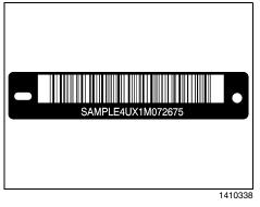
This is the legal identifier for your vehicle. It appears on a plate in the front corner of the instrument panel, on the driver side. You can see it if you look through the windshield from outside your vehicle. The VIN also appears on the Certification/Tire and Service Parts labels and the certificates of title and registration.
