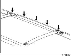
Press the levers down until the locking mechanisms fully engage to the side rail. Make sure each lever is in the down position. The crossrail will not slide when properly engaged.
