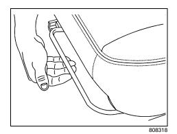
Lift the bar located under the front of the seat to unlock it. Slide the seat to where you want it and release the bar. Try to move the seat with your body to be sure the seat is locked in place.
