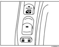
The window switches are located on each side of the shift lever on the center console.
