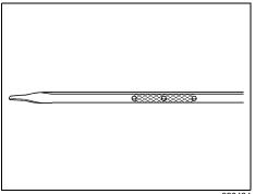
If the oil is below the cross-hatched area at the tip of the dipstick, you need to add at least one quart/liter of oil. But you must use the right kind. This section explains what kind of oil to use. For engine oil crankcase capacity, refer to "Capacities and Specifications" in this section.
