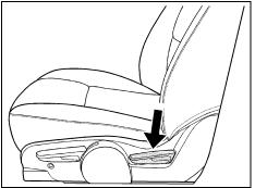
To adjust the seatback on the driver's seat, lift the lever on the rear outboard side of the seat and move the seatback to the desired position. Then release the lever to lock the seatback in place.
