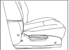
To adjust the seatback on the front passenger's seat, lift the lever on the outboard side of the seat and move the seatback to the desired position. Then release the lever to lock the seatback in place. If your front passenger's seat is a flat folding seat, you must fully raise the lever to disengage the seatback.
