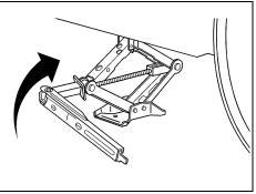
6) Raise the vehicle by turning the jack handle clockwise. Raise the vehicle far enough off the ground so there is enough room for the road tire to clear the ground.
