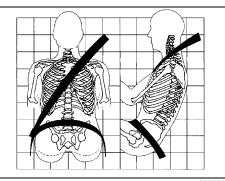
The lap part of the belt should be worn low and snug on the hips, just touching the thighs. In a crash, this applies force to the
