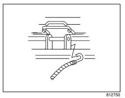
Hook the cable (A) onto the outside of the liftgate hinges (B).
