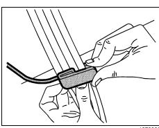
2) Slide the guide under and past the belt. The elastic cord must be under the belt. Then, place the guide over the belt, and insert the two edges of the belt into the slots of the guide.
