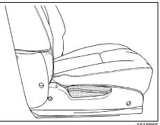
3) Lift the recliner lever, located on the outboard side of the seat, up fully and fold the seatback forward until it disengages.
