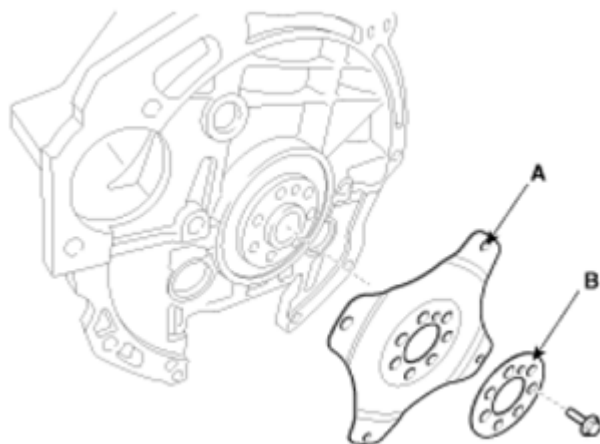
Fig. 44: Identifying Drive Plate Courtesy of HYUNDAI MOTOR CO.
