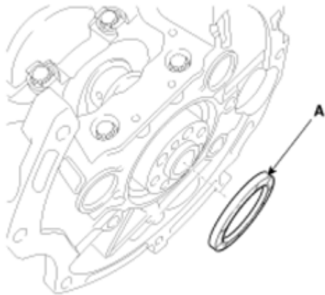
Fig. 5: Identifying Rear Oil Seal Courtesy of HYUNDAI MOTOR CO.
