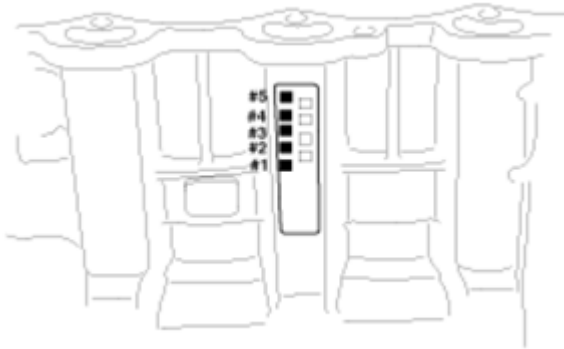
Fig. 15: Identifying Crankshaft Bore Identification Mark Courtesy of HYUNDAI MOTOR CO.
