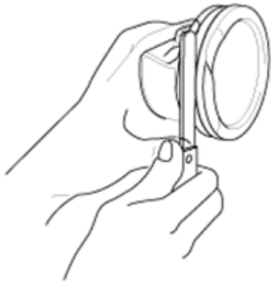
Fig. 25: Checking Piston Ring Side Clearance Courtesy of HYUNDAI MOTOR CO.
