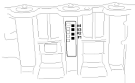
Fig. 22: Checking Cylinder Bore Size Courtesy of HYUNDAI MOTOR CO.
