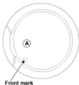
Fig. 23: Checking Piston Size Mark On Piston Top Face Courtesy of HYUNDAI MOTOR CO.
