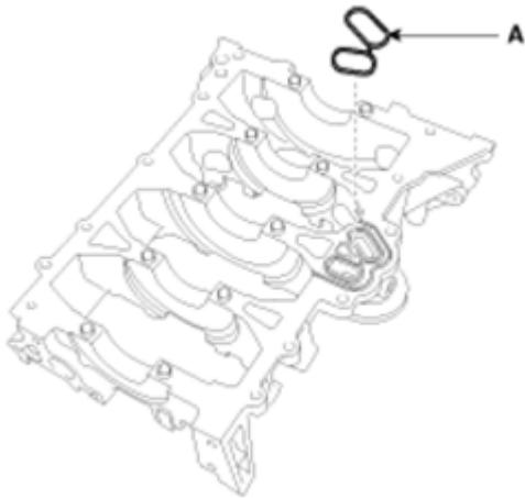
Fig. 35: Identifying Rubber Gasket Courtesy of HYUNDAI MOTOR CO.
