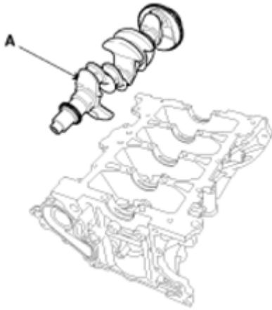
Fig. 34: Identifying Crankshaft Courtesy of HYUNDAI MOTOR CO.
