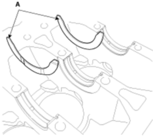
Fig. 33: Identifying Thrust Bearings Courtesy of HYUNDAI MOTOR CO.
