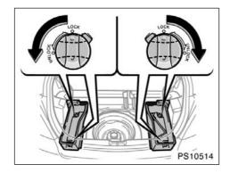
To remove the luggage storage box, turn the knobs to the "UNLOCK" position and remove it.
