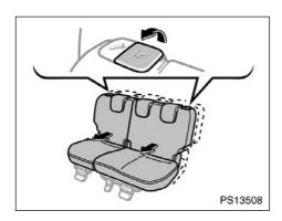
Pull the seat position adjusting liver up. Then slide the rear seat fully forward.
