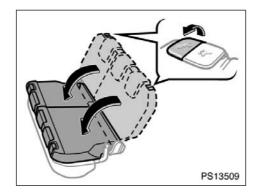
3. Pull the seatback angle adjusting lever up and fold the seatback down.
