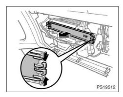
2. Pinch the knobs located on each side and remove the filter cover.
