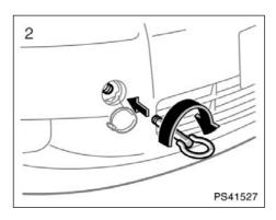
2. Use the towing eyelet in the tool bag. Secure the front towing eyelet to the hole on the front bumper by turning clockwise. (For the tool bag storage location, see "—Required tools and spare tire" on page 230.)
