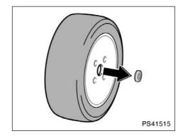
1. Aluminum wheels—Before stowing the flat tire, remove the center wheel ornament by pushing from the reverse side.
