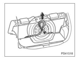
5. Pass the belt through the center hole of the flat tire wheel.
