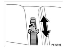
Seat belts with an adjustable shoulder anchor (5-door models)—
