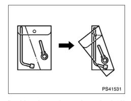
Position the tools as shown in the illustration. Fold the tool bag over and then restow it.
