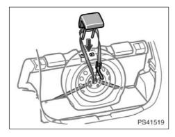
6. Put the center portion of the belt onto the rear center head restraint position and then return the rear center head restraint.
