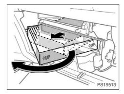
3. Pull out the filter and rotate it as shown in the illustration to remove. Inspect the filter on the surface.
