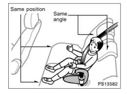
• When installing a child restraint system in the rear seat center position, adjust both seat cushions to the same position and align both seatbacks at the same angle. Otherwise, the child restraint system cannot be securely restrained and this may cause death or serious injuries in a collision.
