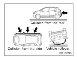
The SRS airbags are not generally designed to inflate if the vehicle is involved in a side or rear collision, if it rolls over, or if it is involved in a low-speed frontal collision. But, whenever a collision of any type causes sufficient forward deceleration of the vehicle, deployment of the SRS airbags may occur.
