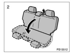
2. Pull the seatback angle adjusting lever up and fold the seatback down.
