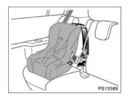
4. Securely fasten the child restraint system with the seat belt.
