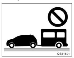
Toyota does not recommend towing a trailer with your Toyota. Toyota also does not recommend the installation of a tow hitch or the use of a tow hitch carrier for a wheelchair, scooter, bicycle, etc. Your Toyota is not designed for trailer towing or for the use of tow hitch mounted carriers.
