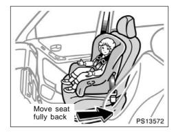
On vehicles with side airbags and curtain shield airbags, do not allow the child to lean his/her head or any part of his/her body against the door or the area of the seat, front or rear pillar or roof side rail from which the side airbags or curtain shield airbags deploy even if the child is seated in the child restraint system. If is dangerous if the side airbag and curtain shield airbag inflate, and the impact could cause death or serious injury to the child.
