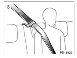
3. Buckle, position and release the seat belt. (For wearing the seat belt, see "—Fastening front and rear seat belts" on page 43 in this Section.)
