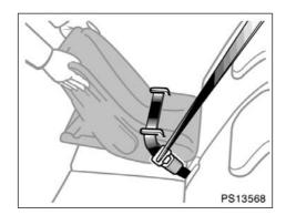
Push and pull the child restraint system in different directions to be sure it is secure. Follow all the installation instructions provided by its manufac-
