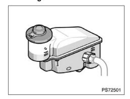
Before checking or adding the brake fluid, remove the cover. (See "(c) Jump starting" on page 223 in Section 4.)
