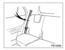
Make sure the outer seat belt passes through the hanger when folding the seatback down.
