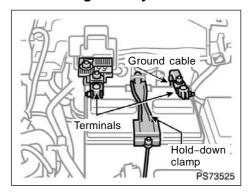
Before checking the battery, remove the cover. (See "(c) Jump starting" on page 223 in Section 4.)
