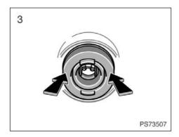
Install the rubber cover as shown and fit it securely on the boss. Plug in the connector.
