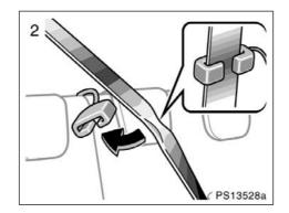
Pinch the two edges of the shoulder belt for the rear seat center position with your fingers and slide the belt past the slot of the guide as shown above. At this time, the elastic cord must be behind the seat belt.
