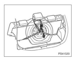
7. Hold the buckle and pull the belt to secure the tire.
