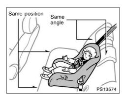
Split seat: When installing a child restraint system in the rear seat center position, adjust both seat cushions to the same position and align both seatbacks at the same angle. Otherwise, the child restraint system cannot be securely restrained and this may cause death or serious injuries in a collision.
