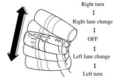
The turn signal indicators (green) in the instrument cluster flash according to the operation of the turn signal lever to show which signal is working.
