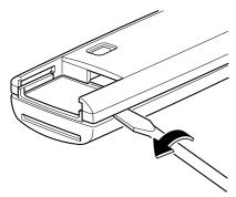
4. Remove the battery cap, then remove the battery.
