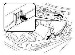
If any fuse but the MAIN fuse is blown, replace it with a new one of the same amperage rating.
