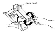
5. Place the jack under the jack-up position closest to the tire being changed with the jack head squarely under the jack-up point.
