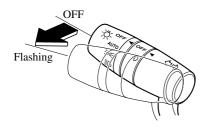
The headlight high-beam indicator light in the instrument cluster illuminates simultaneously. The lever will return to the normal position when released.
