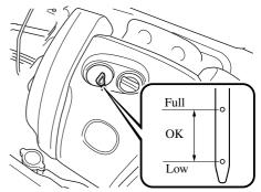
5. Pull it out again and examine the level. The level is normal if it is between Low and Full.
