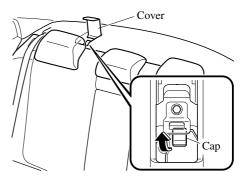
3. Turn the screw counterclockwise and remove it, and then remove the cap.
