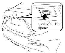
While the ignition is switched ON, the trunk lid can only be opened when the vehicle is stopped.
