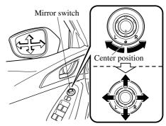
After adjusting the mirror, lock the control by rotating the switch in the center position.
