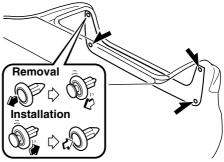
4. Pull the center of each plastic retainer and remove the retainers.
