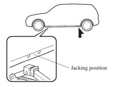
6. Continue raising the jack head gradually by rotating the screw with your hand until the jack head is inserted into the jack-up position.
