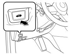
While the ignition is switched ON, the trunk lid can only be opened when the vehicle is stopped.
