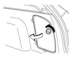
2. Turn the wing bolt and jack screw counterclockwise.
