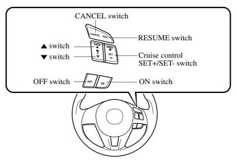
When the system is activated, the vehicle speed and the distance between vehicles while in headway control can be set. The Mazda Radar Cruise Control (MRCC) indication is shown in the active driving display.
