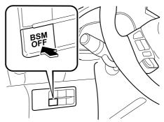
Press the BSM OFF switch again to turn on the BSM system. The BSM OFF indicator light turns off.
