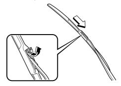
3. Tilt the blade assembly and remove it from the arm.
