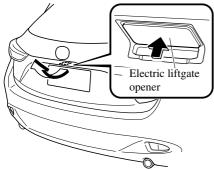
While the ignition is switched ON, the liftgate can only be opened when the vehicle is stopped.
