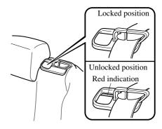
Make sure that the seat belt passes through the seat belt guide correctly and it is not twisted, then raise the seatback while preventing the seat belt from being caught in the seatback. (4-Door)
