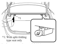
2. Open a rear door and fold the rear seat forward.
