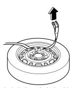
12. Pass the belt through the buckle, then pull the belt end to secure the flat tire.
