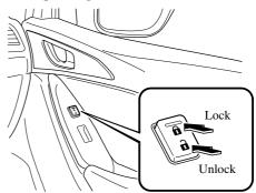
To lock all the doors/liftgate/trunk lid from an open front door, press the lock side of the door lock switch and then close the door.
