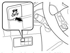
Press the switch again to turn the TCS/DSC back on. The DSC OFF indicator light will turn off.
