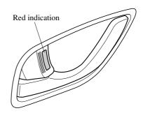
To lock the front passenger door with the door-lock knob from the outside, press the door-lock knob to the lock position and close the door (holding the door handle pulled is not required).
