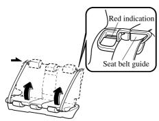
2. Press the seatback rearward and lock it in place. After returning the seatback to its upright position, make sure it is securely locked.
