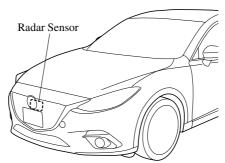
If the Forward Obstruction Warning (FOW) indicator light (amber) is illuminated, the area around the radar sensor may be dirty. Refer to "Warning Guidance" in the type B audio display.
