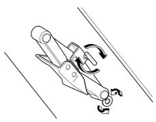
10. Turn the wing bolt completely to secure the jack.
