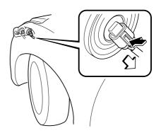
4. Turn the socket and bulb assembly to remove it. Carefully remove the bulb from its socket in the reflector by gently pulling it straight backward out of the socket.
