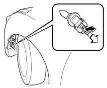
6. Turn the socket and bulb assembly to remove it. Carefully remove the bulb from its socket in the reflector by gently pulling it straight backward out of the socket.
