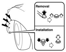
4. Turn the screw counterclockwise and remove it, and then partially peel back the mudguard.
