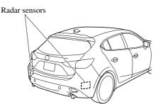
Always keep the bumper surface near the radar sensor area clean so that the BSM system operates normally. Refer to Exterior Care on page 6-63.
