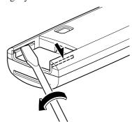
Insert the small, flathead screwdriver into the gap between the cover and the transmitter, and then rotate the screwdriver to detach the cover.
