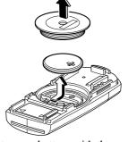
5. Insert a new battery with the positive pole facing up, and then cover the battery with the battery cap.
