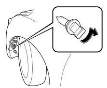
7. Install the new bulb in the reverse order of the removal procedure.
