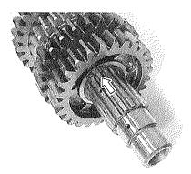
• Remove the washer (6), 4th driven gear (7) and its bushing (8).
