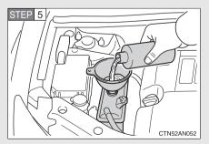
Add engine coolant if necessary.
