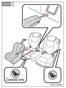
Latch the buckles onto the LATCH anchors.
