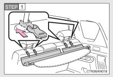
Attach the hooks to the head restraints.
