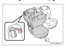
Pull the lever forward and fold down the seatback. The seat will slide forward.
