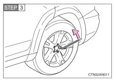
Slightly loosen the wheel nuts (one turn).
