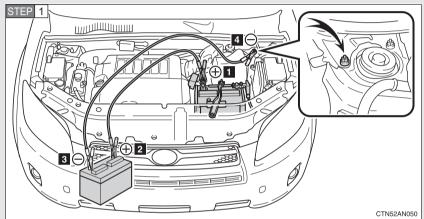
Connecting the jumper cables
