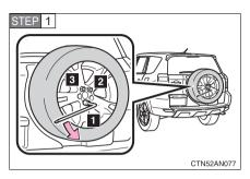
Using the wheel nut wrench, loosen the hold-down nuts by turning them counterclockwise until they can be loosened by hand. Follow the order shown in the illustration.
