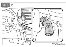
Touch the Toyota emblem side of the electronic kev to "ENGINE START STOP" switch.
