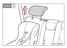
Remove the head restraint.
