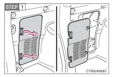
Disengage the claws and remove the cover.
