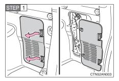
Disengage the claws and remove the cover.
