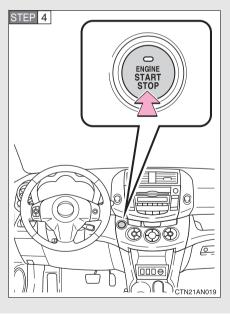
Press the "ENGINE START STOP" switch.
