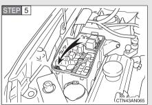
Remove the fuse with the pullout tool.
