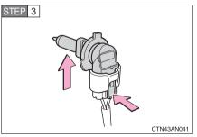
Unplug the connector while depressing the lock release.
