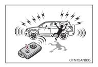
When (i) is pushed for longer than about one second, an alarm will sound for about 60 seconds and the vehicle lights will flash to deter any person from trying to break into or damage your vehicle.
