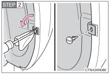
Remove the clip using a flathead screwdriver wrapped in a rag.
