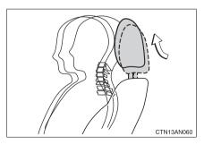
When the occupant's lower back presses against the seatback during a rear-end collision, the head restraint moves slightly forward and upward to help reduce the risk of whiplash on the seat occupant.
