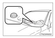
The sensor may not function properly if an object is placed on the sensor, or anything that blocks the sensor is affixed to the windshield.
