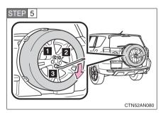
Using the wheel nut wrench, tighten the hold-down nuts by turning them clockwise. Follow the order shown in the illustration.
