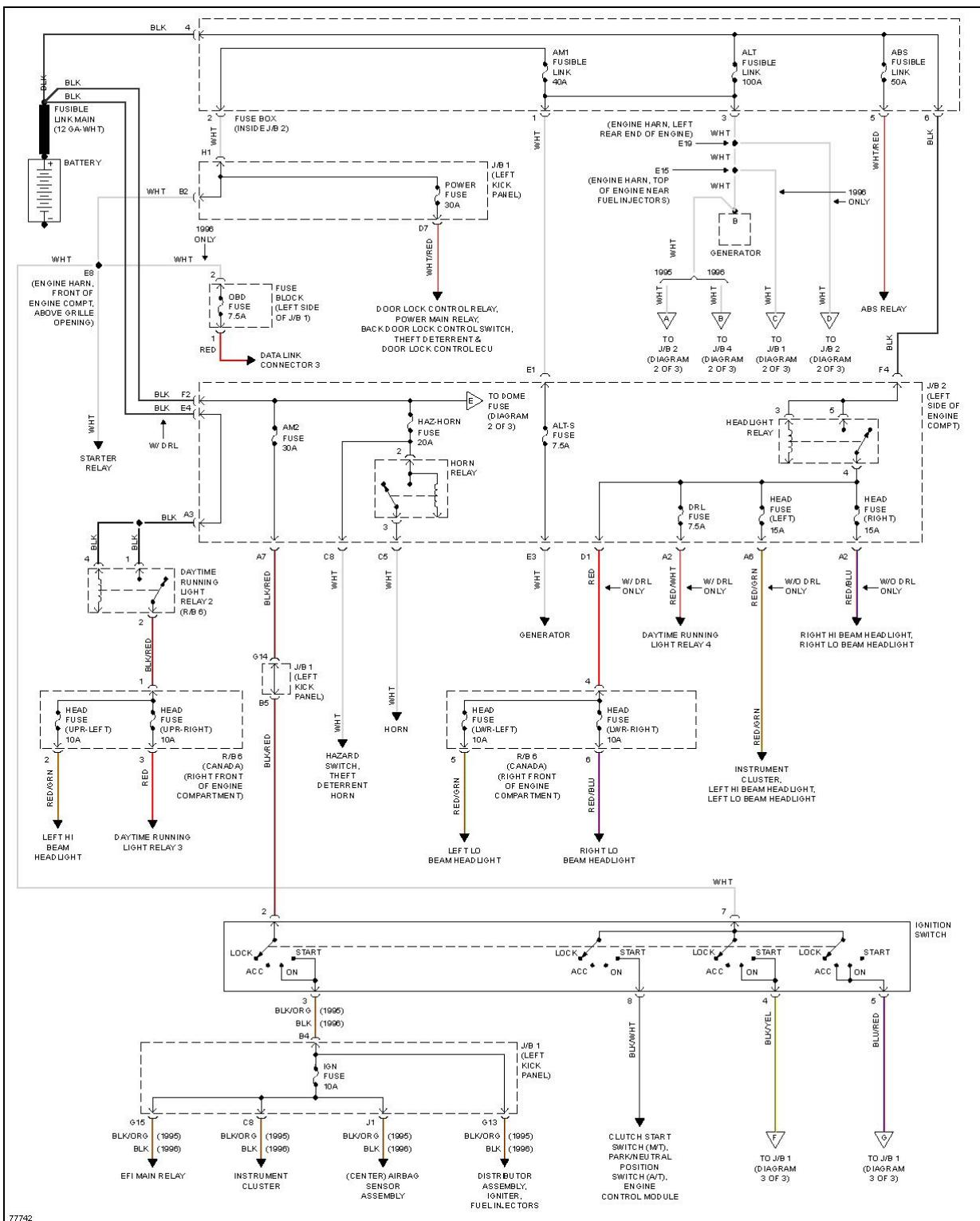
**Fig. 25: Power Distribution Circuit (1 of 3)**
