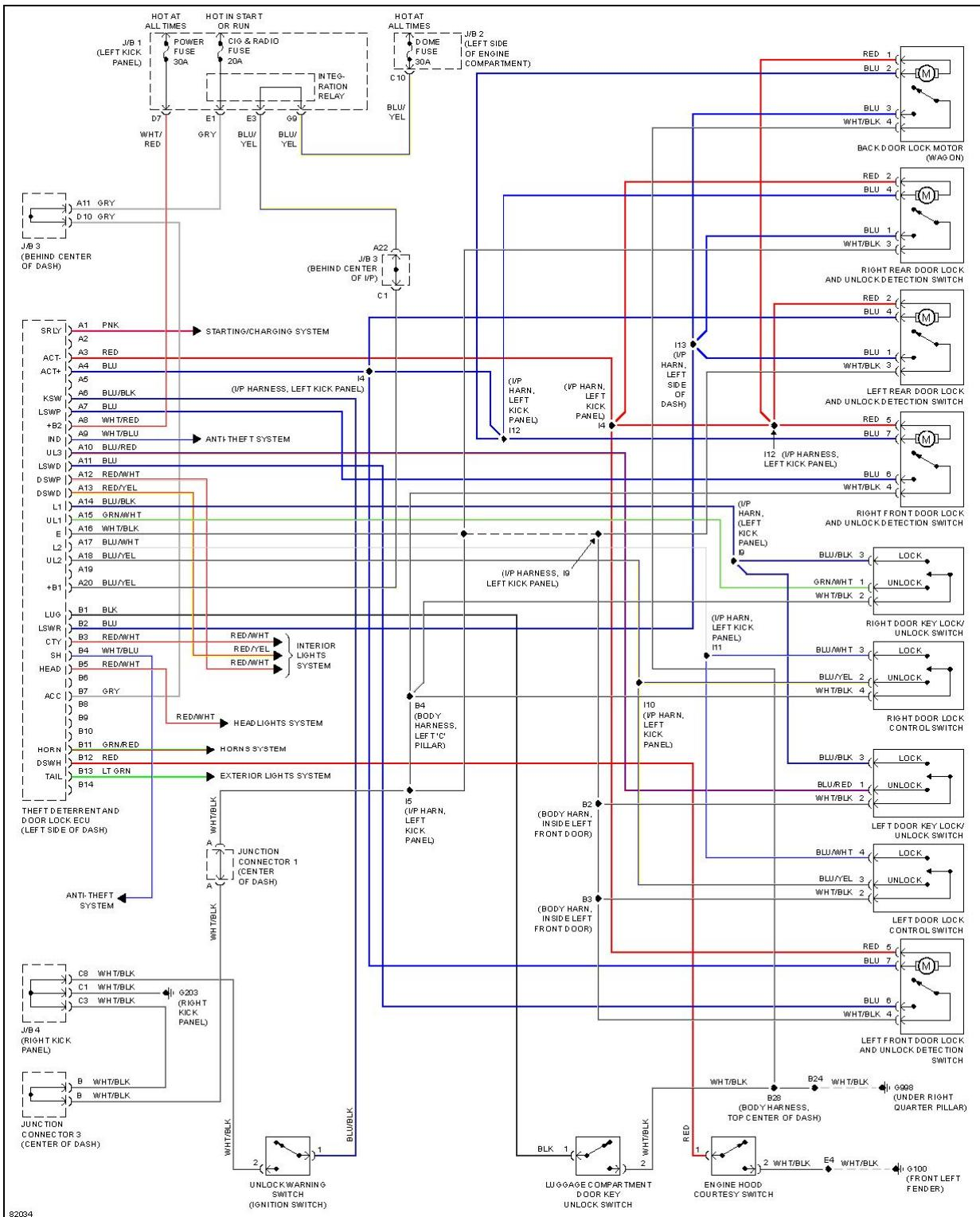
**Fig. 30: Power Door Lock Circuit, Wagon W/ Anti-theft**
