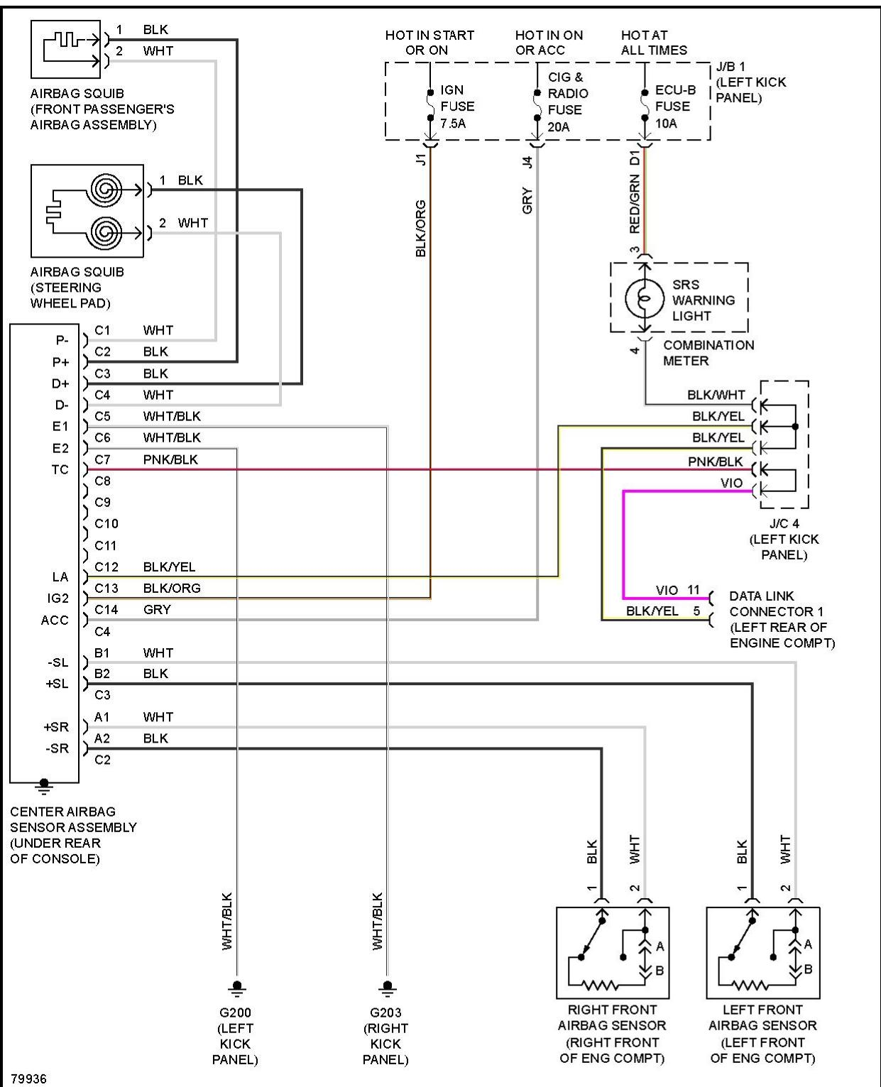
**Fig. 39: Supplemental Restraint Circuit, W/ Front Passenger Airbag Assembly**
