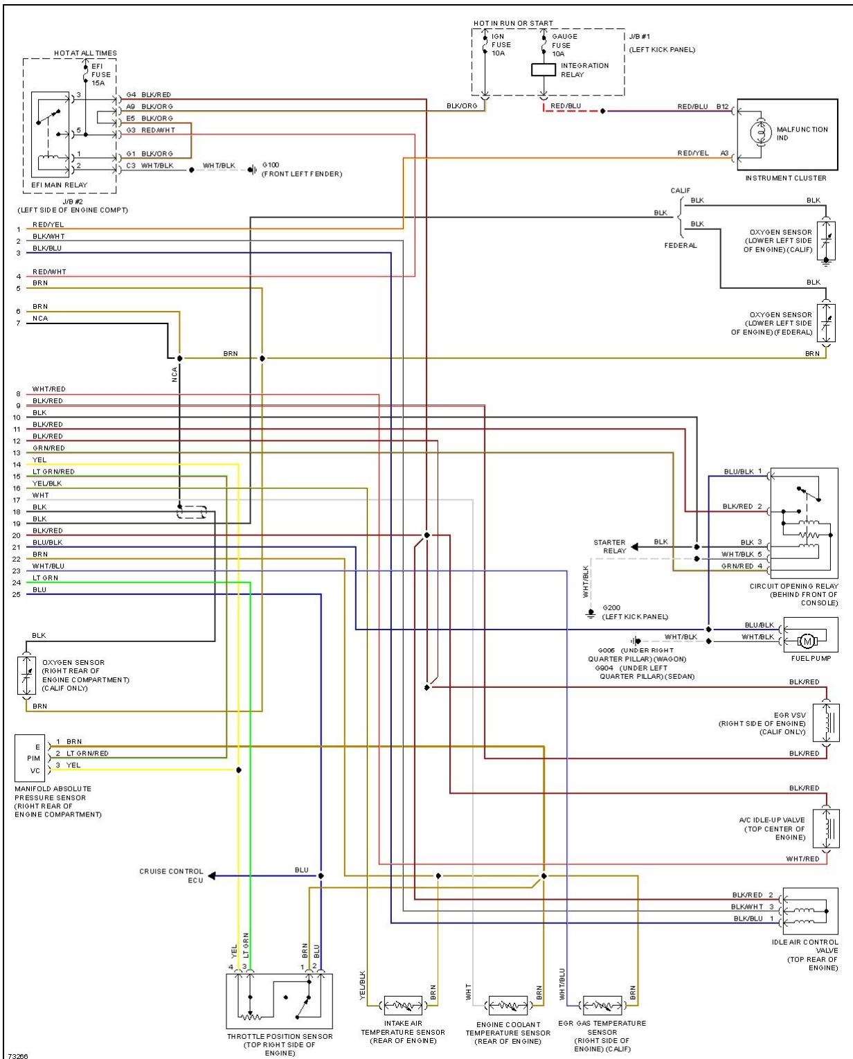
**Fig. 10: 1.6L, Engine Performance Circuits (2 of 2)**
