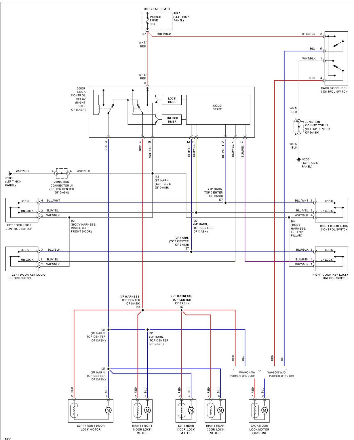
**Fig. 31: Power Door Lock Circuit, Wagon W/O Anti-theft**
