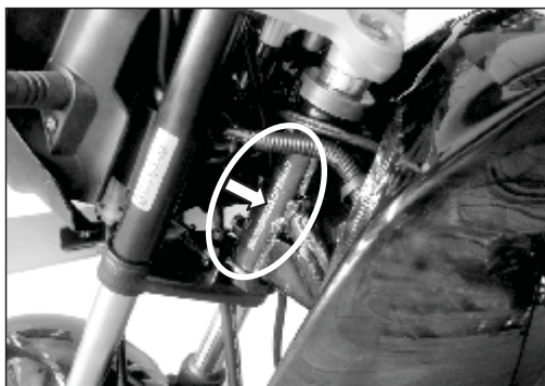
▶ Frame Number Location On LH Side of Steering Tube (Alpha-Numeric - 17 Digits)
