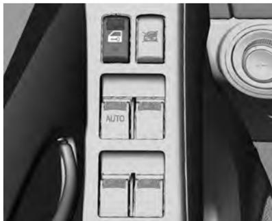
Presione la parte superior del interruptor
