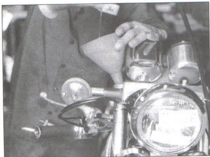
29.7 Use a funnel to pour oil into the fork
