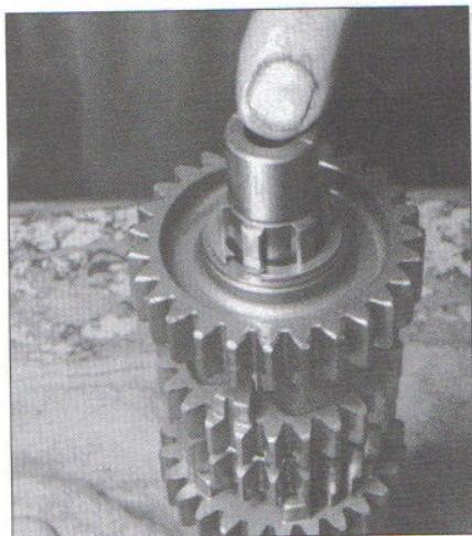
30.11h ...then secure the gear and washer with a snap-ring
