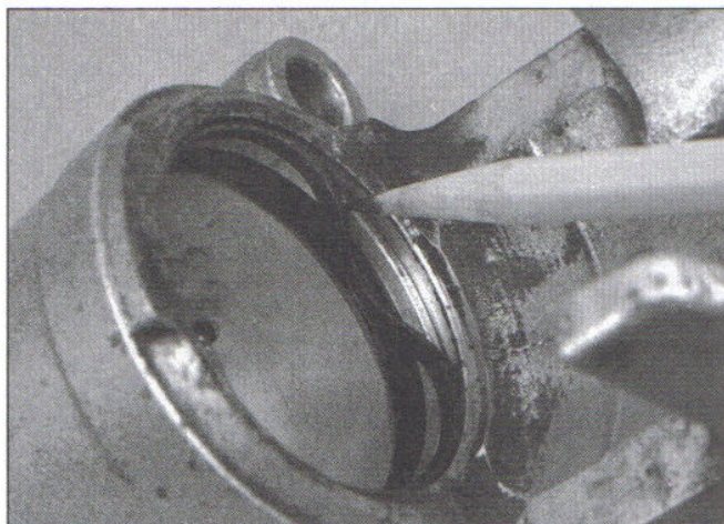
3.9 The dust seal should be removed with a plastic or wooden tool to avoid damage to the bore and seal groove (a pencil works well) - remove the piston seal the same way
