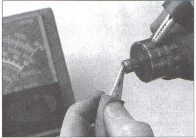
27.8b There should be no continuity between the commutator bars and the armature shaft
