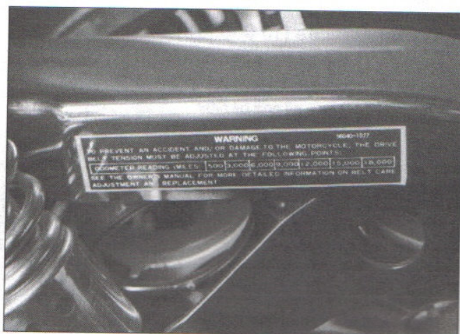
2.3c A decal on the drive belt guard lists belt maintenance intervals
