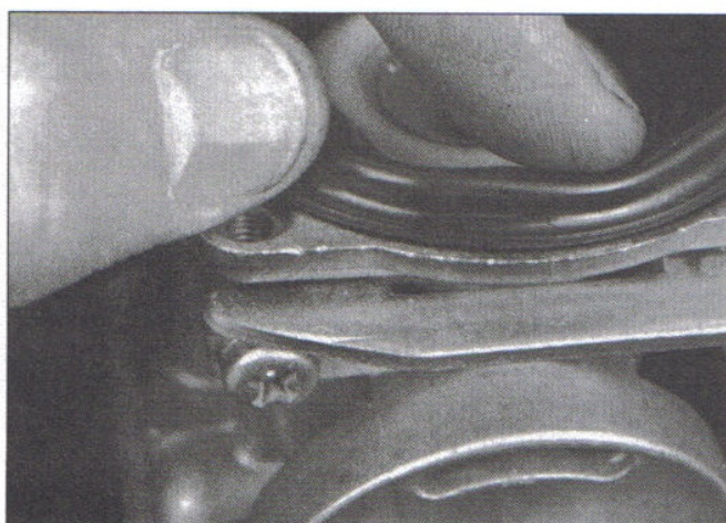
8.8 Make sure the bead of the vacuum diaphragm seats in its groove, and that the diaphragm isn't distorted
