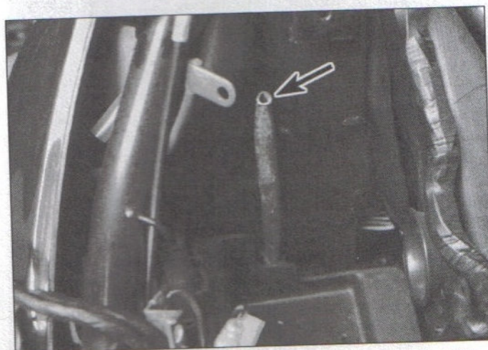
4.11 The clear plastic vent tube supplied with the battery fits inside the motorcycle's drain tube (arrow) when the battery is installed
