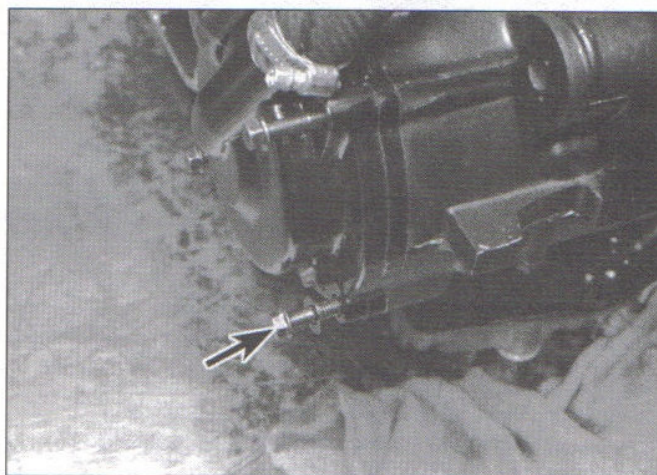
8.19 The lower right cover bolt (arrow) is the only one with a washer
