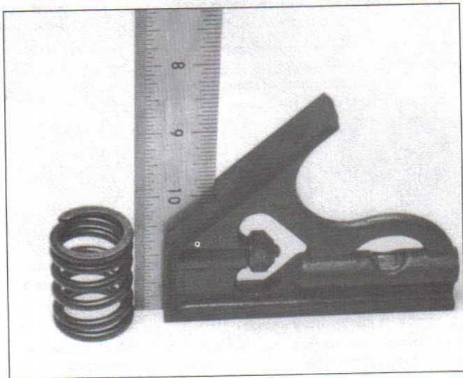
12.19b Check the valve springs for squareness
