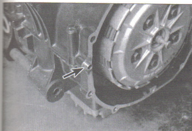
19.5c ...and note the location of the cover dowel
