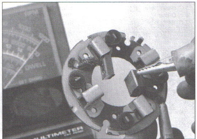
27.9 There should be almost no resistance (0 ohms) between the brushes and the brush plate (EN450 model shown)
