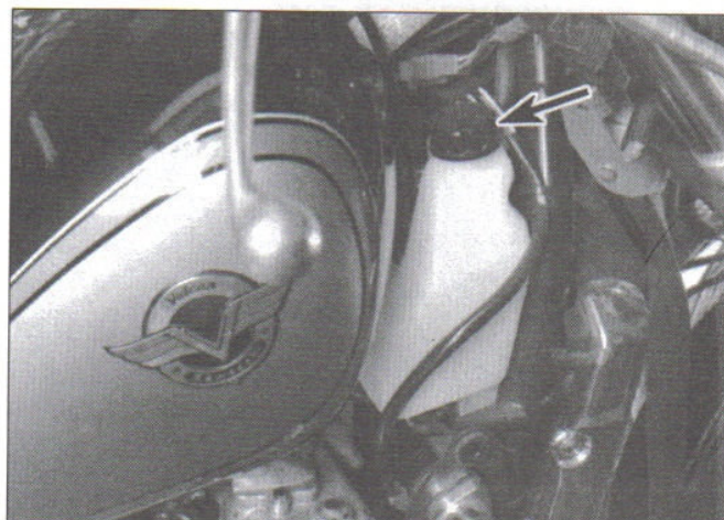
3.16 The reservoir is located inside the right side cover; to add coolant, remove the filler cap (arrow)
