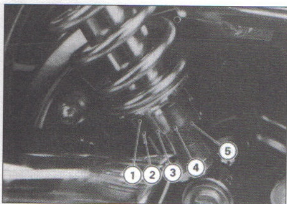
12.2a This is the spring preload adjuster on EN450 models; setting 1 is the softest and setting 5 is the hardest
