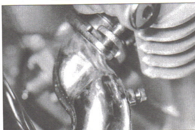
12.10 The holder halves are notched so they form a flush surface when assembled correctly
