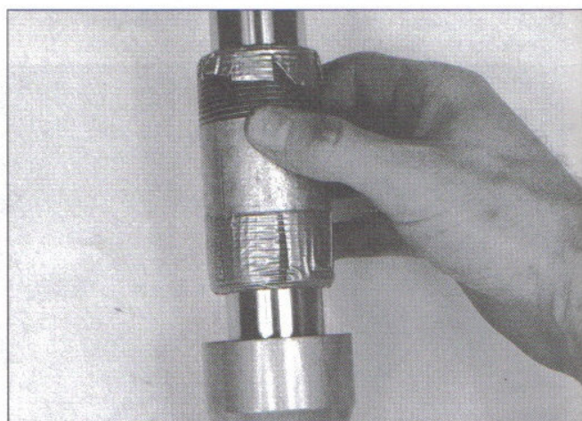
4.18b If you don't have the proper tool, a section of pipe can be used the same way the special tool would be used - as a slide hammer (be sure to tape the ends of the pipe so it doesn't scratch the fork tube)
