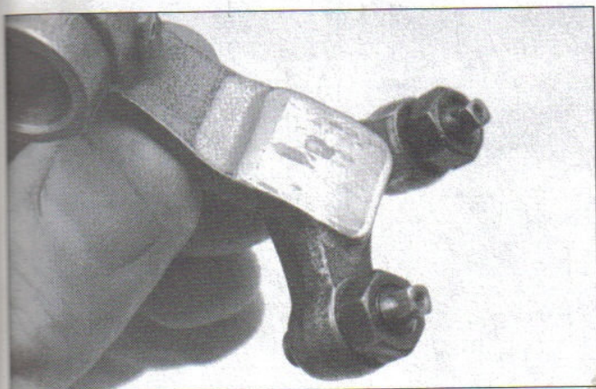
9.33 Inspect the rocker arms, especially the faces that contact the cam lobes, for wear
