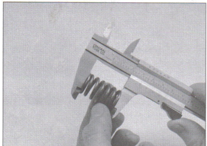
19.11 Measure the clutch spring free length
