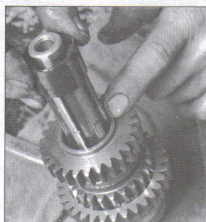
30.15i . . .slide off the bushing and fourth gear
