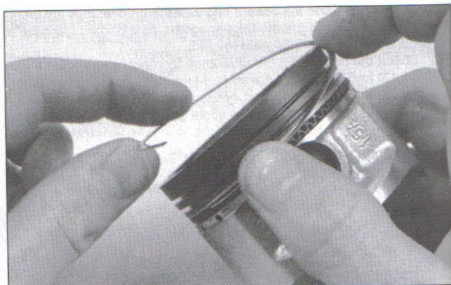
15.9b Installing an oil ring side rail - don't use a ring installation tool to do this
