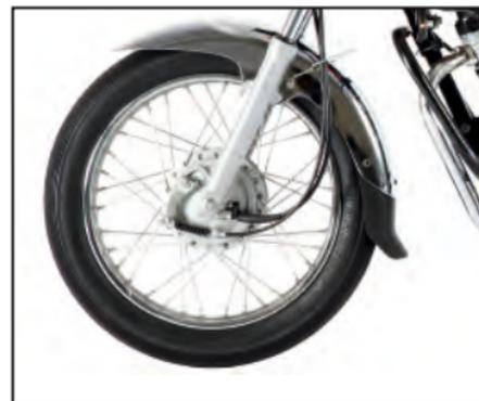
Use the recommended levers while removing the Tyre / Tube for puncture work. This will avoid any damages to the edges / scratches on paint of the wheel.
