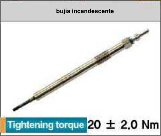
**Tightening torque** 20 ± 2.0 Nm
