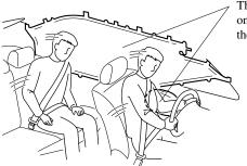
The only one side of curtain air bag will deploy only on the side the vehicle receives the force of the impact.
