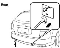
3. Securely install the tiedown eyelet using the lug wrench.
