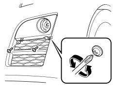
4. Loosen the screws securing the fog light unit.
