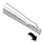
Remove the metal stiffeners from each blade rubber and install them in the new blade.
