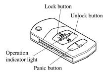
The operation indicator light flashes when the buttons are pressed.
