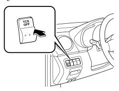
Press the switch again to turn the TCS back on. The TCS OFF indicator light will turn off. If the vehicle speed is more than 30 km/h (18 mph), the TCS OFF indicator light will not illuminate even if the switch is pressed.
