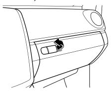
To close the glove compartment, firmly press in the center of the glove compartment lid.
