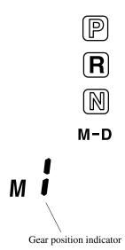
In manual mode, the "M" of the shift position indicator illuminates and the numeral for the selected gear displays in the gear position indicator.
