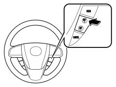
Your vehicle has a tap-up feature that allows you to increase your current speed in increments of 1.6 km/h (1 mph) by a momentary tap of the SET + switch. Multiple taps will increase your vehicle speed 1.6 km/h (1 mph) for each tap.
