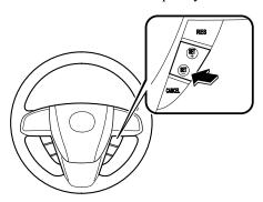
Your vehicle has a tap-down feature that allows you to decrease your current speed in decrements of 1.6 km/h (1 mph) by a momentary tap of the SET- switch. Multiple taps will decrease your vehicle speed 1.6 km/h (1 mph) for each tap.
