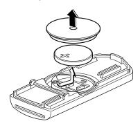
5. Insert a new battery with the positive pole facing up, and then cover the battery with the battery cap.
