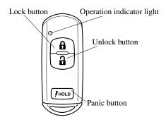
The operation indicator light flashes when the buttons are pressed.
