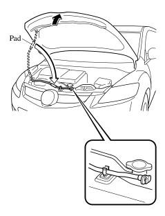
3. Lower the hood slowly until it rests in the unlocked position, and then remove your hands. Push the front center edge of the hood downward until a latching sound is heard, and the hood closes completely.
