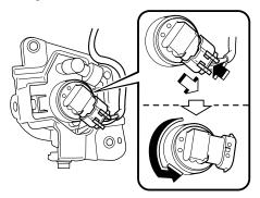
8. Install the new bulb in the reverse order of removal.
