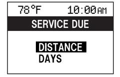
7. Select a digit using the Right switch/ Left switch, and press the Enter (up/ down) switch up or down to change the value of the digit. If there is no need to change a digit, leave it as it is and press the Enter (up/down) switch.
