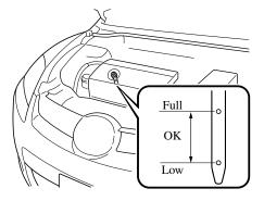
5. Pull it out again and examine the level. The level is normal if it is between Low and Full. If it is near or below Low, add enough oil to bring the level to Full.
