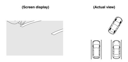
3. When the shift lever is shifted from R to another shift lever position, the screen returns to the previous display.
