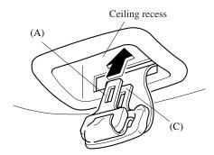
To pull out the seat belt, slide the seat belt tongue (A) with your finger while moving it downward, and slowly pull out the seat belt from the ceiling recess.
