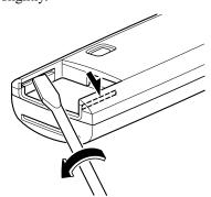
3. Insert the flathead screwdriver into the gap between the cover and the transmitter, and then rotate the screwdriver to detach the cover.
