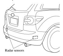
Always keep the bumper surface near the radar sensor area clean so that the BSM system operates normally. Refer to the Exterior Care (page 8-57).
