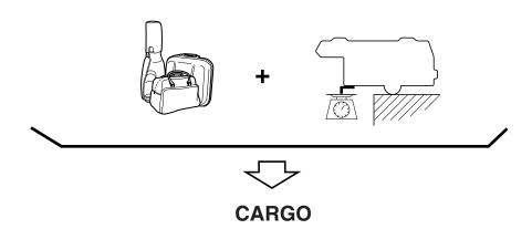
**Cargo Weight** includes all weight added to the Base Curb Weight, including cargo and optional equipment. When towing, trailer tongue load or king pin weight is also part of cargo weight.
