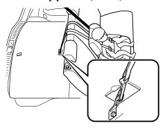
7. Install the head restraint. Refer to Head Restraints on page 2-12.
