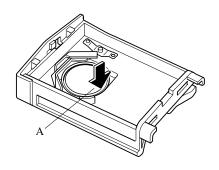
5. Put in the new battery (CR1620 or equivalent) with the positive pole (+) facing down.
