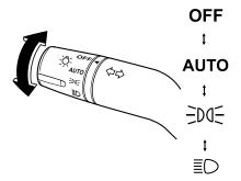
Turn the headlight switch to turn the headlights, other exterior lights and dashboard illumination on or off.
