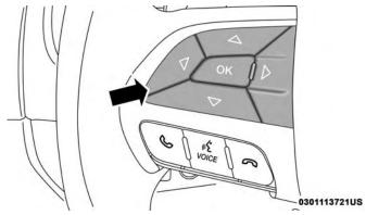
Instrument Cluster Display Controls Up And Down Arrow Buttons:
