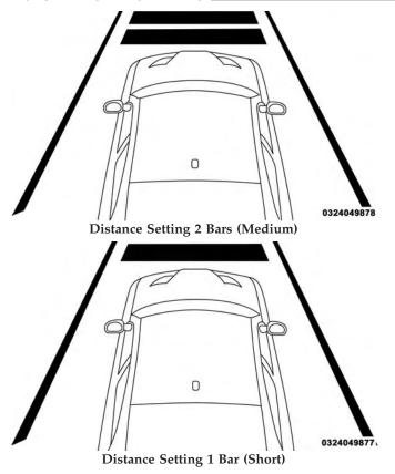
To increase the distance setting, push the Distance Setting — Increase button and release. Each time the button is pushed, the distance setting increases by one bar (longer).
