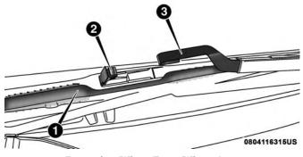
Removing Wiper From Wiper Arm
