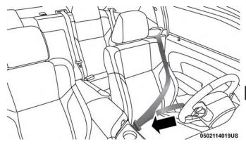
Inserting Latch Plate Into Buckle
