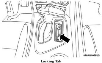
6. While holding the locking tab in the disengaged position, pull the tether strap to rotate the lever up and rearward until it locks in place in the vertical position. The vehicle is now out of PARK and can be moved. Release the parking brake only when the vehicle is securely connected to a tow vehicle.
