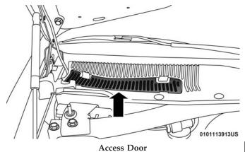
2. Unsnap both ends and lift the filter access cover.
