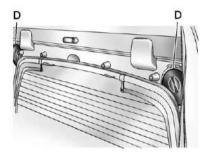
Turn both glass lock knobs (D), located at both top corners of the storage pocket, to the locked position. Push in on the corner of the rear glass to allow the lock knob to engage more easily.
