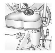
3. Fill the coolant surge tank with the proper mixture to the FULL COLD mark.
