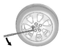
3. Use the wheel wrench to loosen all the wheel nuts. Turn the wheel wrench counterclockwise to loosen the wheel nuts. Do not remove the wheel nuts yet.
