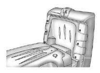
Fold the seatback forward until it is flat. If necessary, move the front seats forward slightly to allow the seatback to fold completely. 4. Repeat the procedure for the other seatback, if desired.
