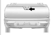
The camera is located under the tailgate handle.
