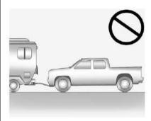
*Notice:* If the vehicle is towed with all four wheels on the ground, the drivetrain components could be damaged. The repairs would not be covered by the vehicle warranty. Do not tow the vehicle with all four wheels on the ground.
