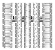
Treadwear indicators are one way to tell when it is time for new tires. Treadwear indicators appear when the tires have only 1.6 mm (1/16 in) or less of tread remaining. Some commercial truck tires may not have treadwear indicators. See *Tire Inspection on page 10-58* and *Tire Rotation on page 10-59* for additional information.
