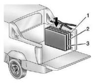
2. Starting with cargo panel 1, load the cargo panel with the latches facing up toward the side of the cargo box.
