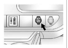
This vehicle has an auxiliary input, located on the audio faceplate, and a USB port located in the center console. External devices such as iPod<sup>®</sup>, laptop computers, MP3 players, CD changers, USB storage device, etc. can be connected to the auxiliary port using a 3.5 mm (1/8 in) input jack or the USB port depending on the audio system.
