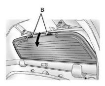
4. With the rear glass tilted at an angle, place the bottom edge in the lower channel of the window frame.
