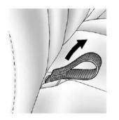
2. Pull the loop in the crease where the seatback and seat cushion meet to release the seat cushion. Tilt the seat cushion forward toward the front of the vehicle. *Notice:* Folding a rear seat with the safety belts still fastened may cause damage to the seat or the safety belts. Always unbuckle the safety belts and return them to their normal stowed position before folding a rear seat.
