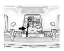
2. Then go to the front of the vehicle and locate the secondary hood release, near the center of the grille.
