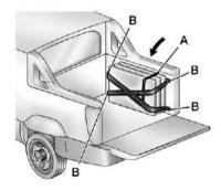
Place the primary straps over the three cargo covers (A). Fasten the four strap clips (B).
