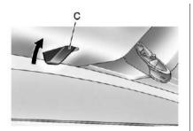
While holding the rear glass in place, press the glass-catch release button (C) and pull the top of the rear glass toward you using the grab handles (B) located at the top of the rear glass.
