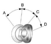
The ignition switch has four different positions.
