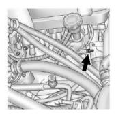
The remote negative (-) terminal is a stud located on the right front of the engine, where the negative battery cable attaches.
