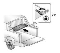
The driver side cargo cover panel latch must lock in place before the passenger side latch can be locked. If this procedure is not followed exactly, the cargo cover panels might not correctly lock in place. Push the driver side latch toward the front of the vehicle to lock the cover in position. A click sounds when
