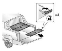
2. Unlock the cargo panel 3 by pulling forward on the driver side and passenger side cargo panel latches, located on the bottom of each cargo panel.
