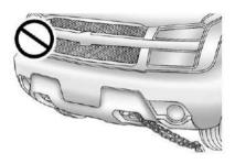
*Notice:* Never use recovery hooks to tow the vehicle. Your vehicle could be damaged and it would not be covered by warranty.
