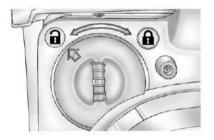
2. Hold the rear glass in place with one hand and turn the glass lock knobs, located at both top corners of the glass storage pocket, to the unlocked position. 3. Pull the rear glass out from the storage pocket using the grab handles (B).
