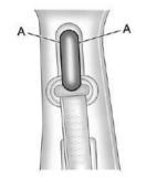
Squeeze the buttons (A) on the sides of the height adjuster and move the height adjuster to the desired position.
