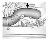
4. With the coolant surge tank pressure cap off, start the engine and let it run until the upper radiator hose can be felt getting hot. Watch out for the engine cooling fan. By this time, the coolant level inside the coolant surge tank may be lower. If the level is lower, add more of the proper mixture to the coolant surge tank until the level reaches the FULL COLD mark.
