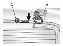
2. Squeeze and pull down the latch levers (A), located near the upper corners of the rear glass, to unlatch. Once unlatched, the glass-catch release button (C) will catch the rear glass and prevent it from falling forward.
