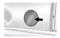
The tethered fuel cap is located behind a hinged fuel door on the driver side of the vehicle. If the vehicle has E85 fuel capability, the fuel cap will be yellow and state that E85 or gasoline can be used. See *Fuel E85 (85% Ethanol) on page 9-59.*
