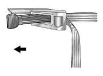
5. Close both cross locks at the center of the strap system to tightly secure.
