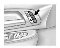
On vehicles with the memory feature, the controls on the driver door are used to program and recall memory settings for the driver seat, outside mirrors, and the adjustable throttle and brake pedals, if equipped.
