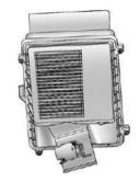
2. Loosen the four screws on the cover of the housing and lift up the cover.
