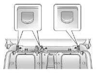
The top tether anchors are located on the back of the rear seat frame above the floor for each rear seating position. Fold down the rear seatback(s) to access the anchors.
