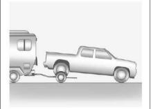
Two-Wheel-Drive Vehicles and Four-Wheel Drive Vehicles with a Single Speed Automatic Transfer Case Use the following procedure to dolly tow the vehicle from the rear:
