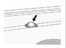
The solar sensor, located in the defrost grille, middle of the instrument panel, monitors the solar heat. Do not cover the solar sensor or the system will not work properly.
