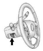
The tilt lever is located on the lower left side of the steering column.
