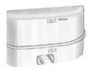
The fluid level should be above MIN. If it is not, have the brake hydraulic system checked to see if there is a leak. After work is done on the brake hydraulic system, make sure the level is above the MIN but not over the MAX mark.
