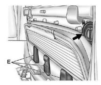
Load the rear glass into the storage pocket in the Midgate, guiding the lower edge of the rear glass behind the three rear glass retaining tabs (E).
