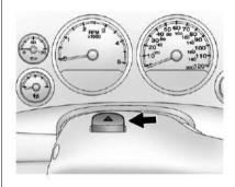
(Hazard Warning Flashers): Press this button located on top of the steering column, to make the front and rear turn signal lamps flash on and off. This warns others that you are having trouble. Press again to turn the flashers off. When the hazard warning flashers are on, the vehicle's turn signals will not work.
