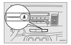
When the key is turned to the "ON" position, this indicator normally comes on and goes off a few seconds later.
