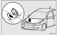
Support the engine hood with the hood prop. Insert the hood prop securely in the opening under the hood marked with an arrow.
