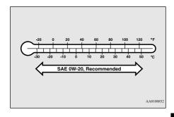
SAE 0W-20 engine oil is strongly recommended for optimum fuel economy and cold starting.
