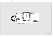
4. The headlights will come on in the low beam setting for about 30 seconds. After the headlights go off, the headlights can be turned on again in the low beam setting for about 30 seconds by pulling the turn signal lever toward you within 60 seconds of turning the ignition switch to the "LOCK" position. To turn on the headlights again after 60 seconds of turning the ignition switch to the "LOCK" position, repeat the process from step 1.
