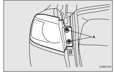
2. Remove the light unit in the rear direction.
