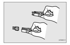
4. Use the fuse location diagrams and the matching tables, to check the fuse that is related to the problem. If the fuse is not blown, something else must be causing the problem. Contact an authorized Mitsubishi Motors dealer or a repair facility of your choice to have the problem checked
