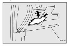
2. For vehicles with the bottom cover, use the puller to loosen the 2 clips (A) and push down the bottom cover. The puller is in the fuse block in the engine compartment. Refer to "Fuse replacement" on page 9-32.
