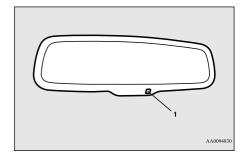
Normally, use the automatic mode. When the ignition switch is turned to the "ON" position, the reflection factor of the mirror is automatically changed.
