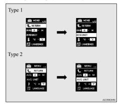
3. Press and hold the multi-information meter switch (for about 2 seconds or more) to display "AVG UNIT" (fuel consumption display unit setting).
