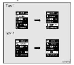
Press and hold the multi-information meter switch (for about 2 seconds or more) to change in sequence from °F → °C → °F.
