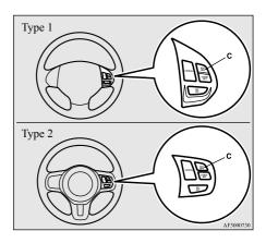
To increase the speed in small amounts, press the "ACC RES" switch (C) for less than 1 second and release it. Every time you press the "ACC RES" switch (C), the speed will increase by approximately 1 mph (1.6 km/h).
