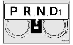
In addition, when the vehicle is driven with the gearshift lever in the "D" (DRIVE) position, the forward gear number is shown.
