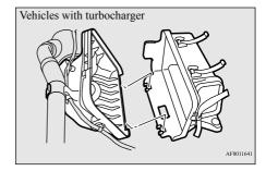
5. Put the duct back on in its original position.
