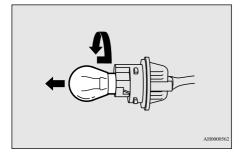
5. To install a bulb, perform the removal steps in reverse.
