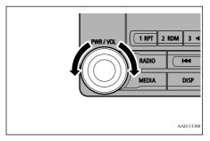
Turn the PWR/VOL key clockwise to increase, and counter- clockwise to decrease the volume.
