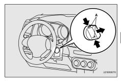
3. Insert the emergency key into the ignition switch.
