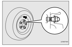
• Compact spare wheel Install the wheel nuts with their tapered ends facing inward, then tighten by hand until the wheel is no longer loose.
