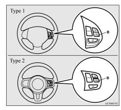
To decrease the speed in small amounts, press the "COAST SET" switch (B) for less than 1 second and release it. Every time you press the "COAST SET" switch (B), the speed will decrease by approximately 1 mph (1.6 km/h).
