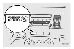
The indicator normally comes on when the ignition switch is turned to the "ON" position and goes out a few seconds later.
