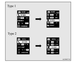
Press and hold the multi-information meter switch (for about 2 seconds or more) to display "ALARM" (rest time setting).
