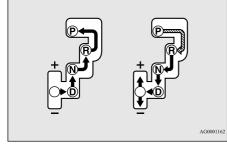
With the brake pedal depressed, set the selector lever in the gate to operate.
