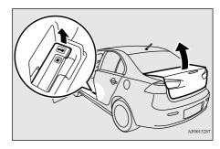
Pull the trunk lid release lever, located to the left of the driver's seat, up to open the trunk.
