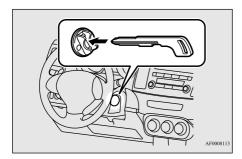
4. Insert the first valid F.A.S.T.-key into the emergency key.
