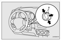
3. Insert the emergency key into the ignition switch, and slowly push and turn.
