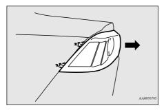
3. Remove the socket and bulb assemblies by turning them counterclockwise.
