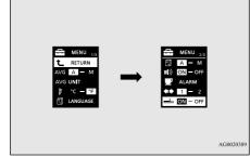
3. Press and hold the multi-information meter switch for about 2 seconds or more to switch in sequence from ON (with the green bar graph)  $\rightarrow$  OFF (without the green bar graph)  $\rightarrow$  ON (with the green bar graph).
