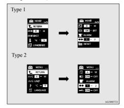
3 Press and hold the multi-information meter switch for about 2 seconds or more to switch in sequence from 1 (turn signal sound 1)  $\rightarrow$  2 (turn signal sound 2)  $\rightarrow$  1 (turn signal sound 1).
