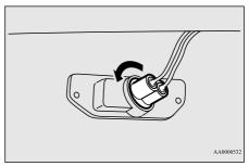
3. Remove the bulb by pulling it out.
