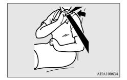
3. Pull the seat belt out slowly while holding the latch plate. Push the latch plate into the buckle until you hear a "click". Pull up on the belt to be sure the latch plate is locked securely in the buckle.
