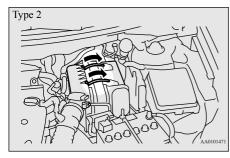
4. Install the air cleaner filter and put the cover back on in its original position.
