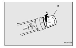
The wipers will operate once if the lever is moved to the "AUTO" position and the knob
