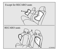
A label is attached to the seatbacks in vehicles with side airbags.
