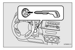
4. Insert the F.A.S.T.-key into the emergency key.
