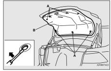
2. Remove the socket and bulb assemblies by turning them counterclockwise.
