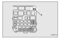
Clamp it on the fuse you wish to remove, and pull the fuse straight out from the fuse block.
