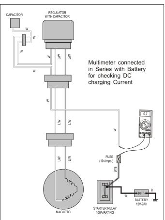
Battery DC Charging current : (Use fully charged battery ensuring battery voltage =  $12.5 \pm 0.3 \text{ V}$  before measuring)
