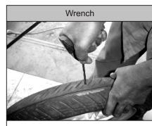
Step 1: Identify the puncture hole & pearse the wrench.
