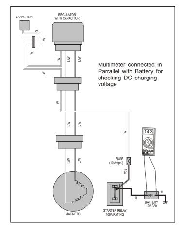
DC Charging Voltage Measurement : (Use fully charged battery while measuring)
