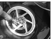
Dip the wheel assly into water and confirm for leakage between tyre & rim.
