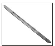
Carefully press the tyre bead portion with crowbar to fit the bead portion in the wheel rim.
