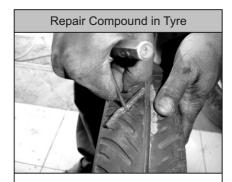
Step 2 : Pearse the repair compound into the puncture hole with needle type wrench.
