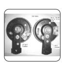
Do not hit by mallet / screw driver on horn resonator.
