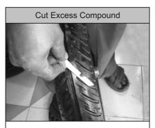
Step 3: Cut the excess compound with blade.
