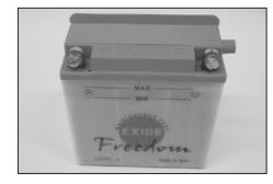
DC Ignition System works on DC electrical energy given by battery. The vehicle battery is always kept charged by the magneto through DC voltage regulator which is incorporated in the R.R. unit. Hence the role of the battery is very important and you can not disconnect the battery from the vehicle. Disconnection of the battery will disable the starting of the vehicle.
