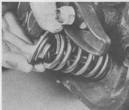
48.5 Installing the valve retainer
