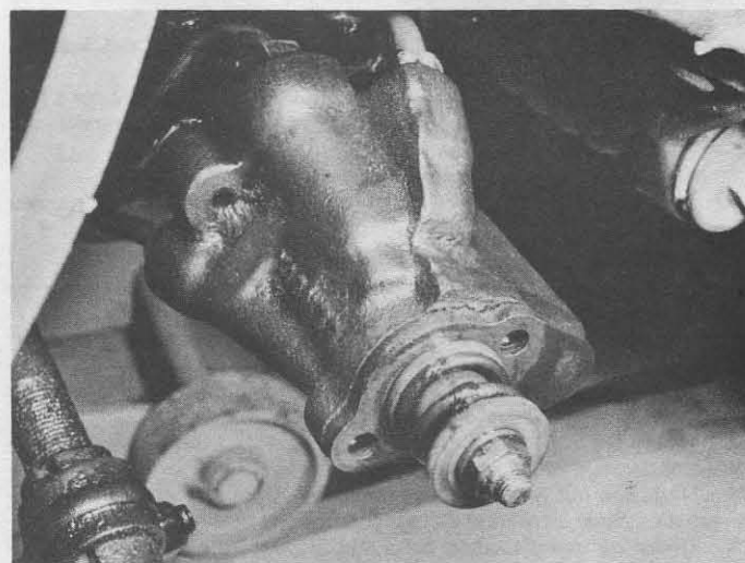
24.2 Non-integral power steering control valve with spring cap removed
