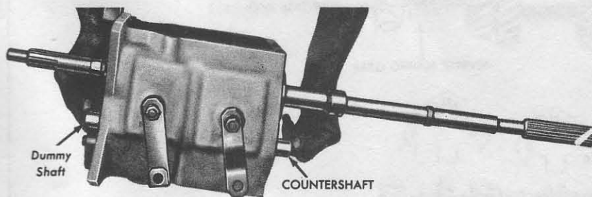
Fig. 6.8 Removing the countershaft (3-speed) (Sec. 3)
