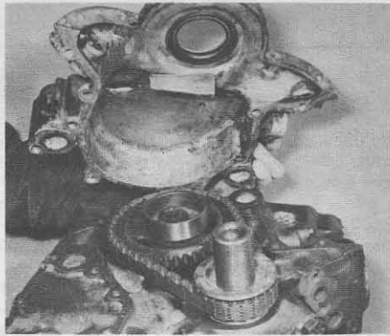
46.9 Lowering the timing cover into position
