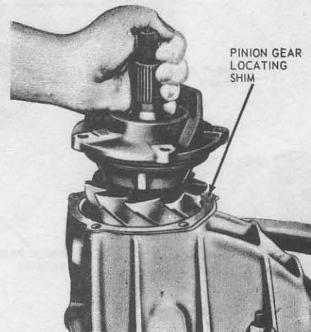
Fig. 8.10 Installing the pinion gear and retainer (Sec. 8)
