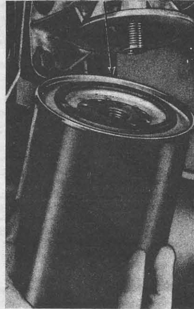
Fig. 1.23 Installing a new oil filter (Sec. 27)
