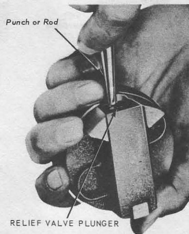
Fig. 11.28 Cleaning the power steering pump relief valve (Sec 22)
