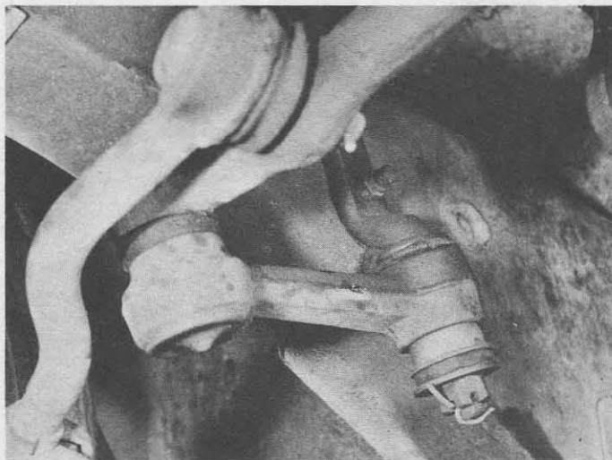
41.3 Steering linkage idler arm removal
