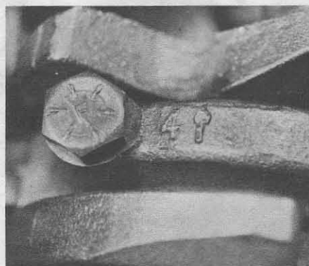
44.12 Identification mark on main bearing cap
