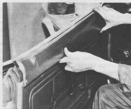
10.12 Fitting the trim panel on the door
