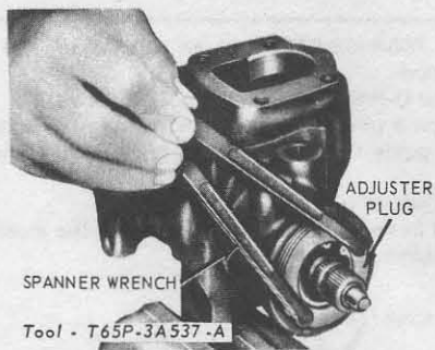
Fig. 11.50 Removing the adjuster plug (Sec 30)
