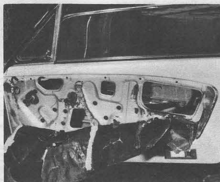
10.4 Door with trim panel removed and watershield pulled back
