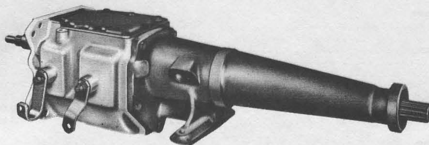
Fig. 6.1 3-speed transmission (Sec. 1)
