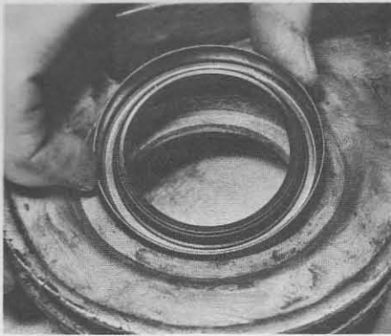
46.8 Installing the timing cover oil seal
