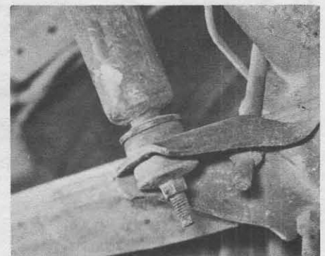
12.1 Rear shock absorber lower mounting
