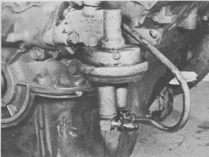
7.1 Disconnecting the fuel lines at the fuel pump
