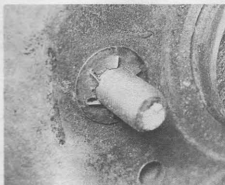
11.2A One of the Tinnerman type nuts securing the brake drum
