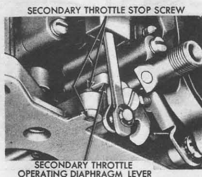
Fig. 3.42 Adjusting the secondary throttle plate (Holley 4150C carburetor) (Sec. 17)
