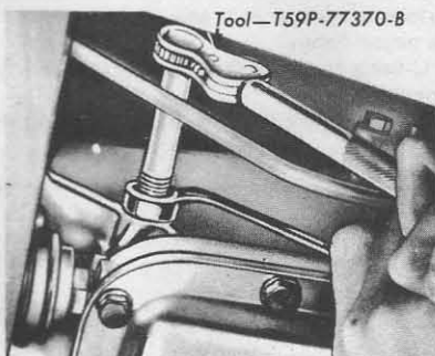
Fig. 6.44 Adjusting low (reverse band) (Sec. 36)
