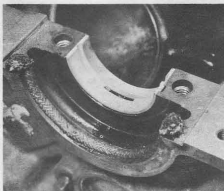
44.6 Installation of rear main bearing and oil seal
