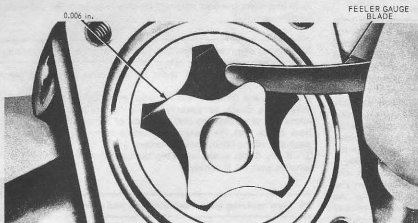
Fig. 1.29 Checking the oil pump inner rotor lobe clearance (Sec. 40)
