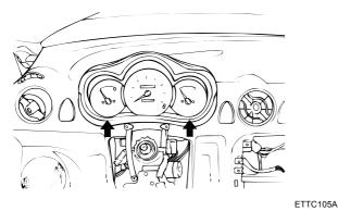
3. Remove the instrument cluster mounting screws.
