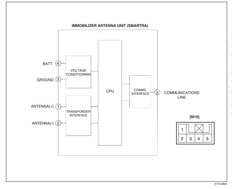
When the key is inserted in the ignition and turned to the ON position, the immobilizer antenna unit sends power to the transponder in the ignition key. The transponder then sends a coded signal back through the immobilizer antenna unit to the ECM/PCM.
