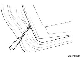
5. Remove the door trim seal and lower the window glass.
