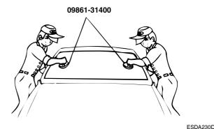
11. Perform a water-leak test for the tailgate glass. Use a cold water spray, being careful not to direct a powerful stream of water on the new adhesive material. Allow water to spill over the edges of the glass.
