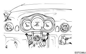
8. Remove the crash pad mounting bolts and disconnect the connectors.
