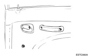
Remove the safety lock rod knob. З.
