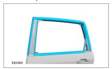
10. NOTE: The rear door window glass must be removed towards the outside of the window opening.
