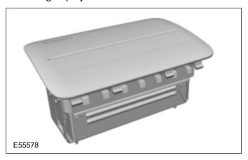
The passenger air bag module is located above the glove compartment and is secured to the in-vehicle crossbeam and the instrument panel. The cover is integrated into the instrument panel to provide an unobtrusive appearance. The cover has invisible 'split lines' moulded in its surface allowing the air bag to easily exit through the cover when the system deploys.
