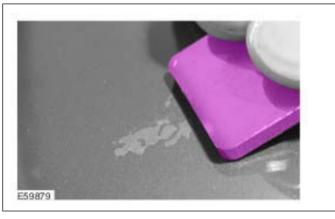
This tool allows paint faults to be carefully removed in shavings. Afterwards the surface must be polished using suitable materials.
