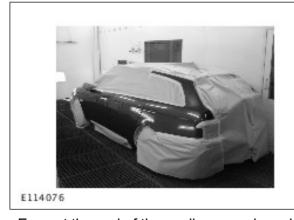
Even at the end of the sealing area, by painting with the masking tape folded up as shown in the figure, it is possible to make the steps far less conspicuous.
