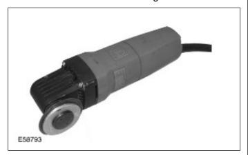
In addition the cut can be made to an exact depth limit. This prevents damage to underlying components.
