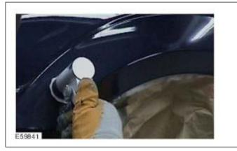
Minor damage can be removed with a small sanding machine or preferably with an eccentric sander with P1500 - P2000. Very fine spray mist
