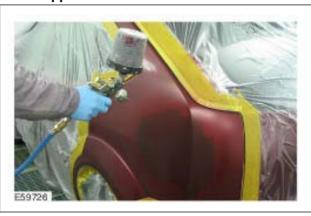
The base paint is applied in two or three steps. First of all only the repair area is painted with the first paint application.
