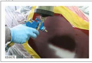
Filler can now be applied to the dried repair area. Choose the correctly toned filler according to the manufacturer's instructions.
