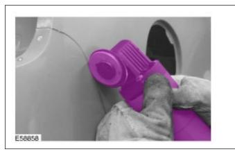
The cutting depth of the orbital saw can be set. This allows separating cuts to be made, despite panels or other components lying in danger behind. Straight cut lines can be more easily made using the orbital saw.
