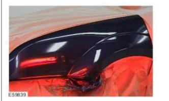
Now dry the clear lacquer according to the manufacturer's instructions using an infrared gun.
