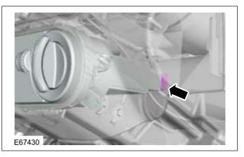
18. Remove the instrument panel (vehicles without passenger airbag view shown).
