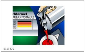
3. Painting with a spatula and color comparison. Test-paint the mixed color on a test plate and confirm whether or not it is the correct color after it dries.
