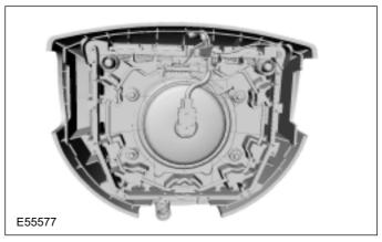
The driver air bag module is fitted to the steering wheel, the cover forming the outer surface of the steering wheel boss. The cover has invisible 'split lines' moulded in its surface allowing the air bag to easily exit through the cover when the system deploys. A new driver air bag module and driver air bag module wiring harness must be installed following deployment.
