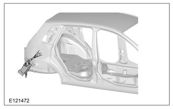
5. Remove tiny wrinkles caused by the shrinkage by hitting them lightly with a hammer and dolly.
