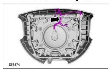
3. Remove the driver air bag module wiring harness.
