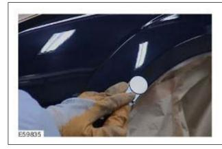
Sand out the damaged location using P180 - P320. Only small sanding blocks and small sanding machines must be used, so that the area of the repair remains as small as possible.
