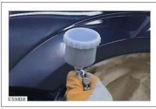
Before painting, clean the area for the final time using a dust-bonding cloth. Then apply the basic paint in thin layers using a spray gun until enough coverage is achieved.
