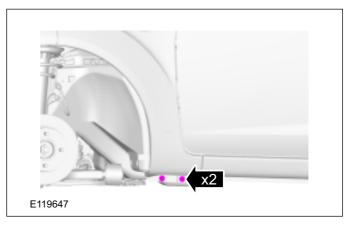
11. Remove the fender front retaining bolts.
