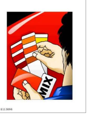
2. Select primary colors. Comparing with the body color, select the most appropriate colors of which direction, hue, and other factors are close to the body color. At the same time, confirm their roughness of metallic or pearl base particles and their brightness.
