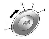
The ignition switch has four different positions.
