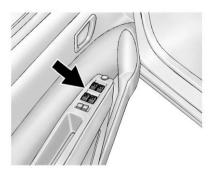
The switches on the driver door control all windows. In addition, each passenger door has a switch for its own window.
