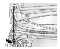
Securely place the hood prop into the hood prop holder, at the rear passenger side of the engine compartment. To close the hood:
