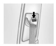
To move it down, press the release button and move the height adjuster to the desired position.
