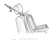
If the rear outboard seating position you are using has an adjustable head restraint and you are using a single tether, raise the head restraint and route the tether under the head restraint and in between the head restraint posts.
