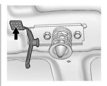
Go to the front of the vehicle and push the secondary hood release lever up.
