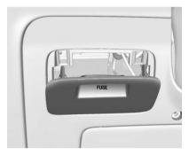
Open the fuse panel door by pulling out at the top.
