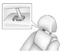
The vehicle has a shopping bag hook under the front seat head restraints. Lift the head restraints to access the hook.
