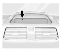
The indicator light on the center stack, indicates the status of the system.
