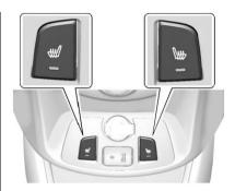
If available, the buttons are below the climate control system. To operate, the engine must be running.
