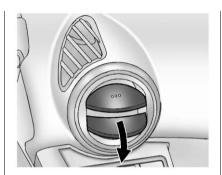
Press the cover of the side air vents to open. Turn open slats clockwise or counterclockwise to direct airflow as needed. Close the cover to stop the airflow.
