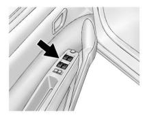
Press the switch down to open the window. Pull the front of the switch up to close it.
