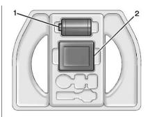
2. Remove the tire sealant canister (1) and the compressor (2).
