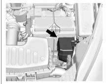
The auxiliary fuse block is located on the driver side of the vehicle, near the battery.
