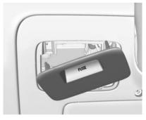
Remove the fuse panel door diagonally.
