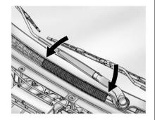
The air intake at the base of the windshield inside the engine compartment must be kept clear to allow the flow of air into the vehicle. Clear away any ice, snow, or leaves.
