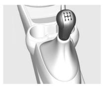
Notice: Shifting the vehicle initially into any gear other than 1 (First) or R (Reverse) can damage the clutch. Shift the manual transmission in the proper sequence, and time the gear shifting with the accelerator to avoid revving the engine and damaging the clutch.
