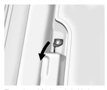
The tethered fuel cap is behind a hinged fuel door on the passenger side of the vehicle. To open the fuel filler door, lift the fuel door release lever on the floor, left front side of the driver seat. The fuel door is unlocked when the vehicle is unlocked. Locking the vehicle locks the fuel door.
