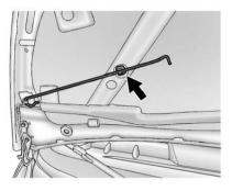
3. Lift the hood and release the hood prop from the prop retainer, which is under the hood.
