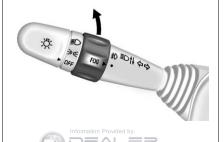
For vehicles with fog lamps, they are controlled by the ‡0 band on the middle of the turn signal lever.
