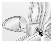
If equipped, move the control up. down, or side to side to adjust the mirror.
