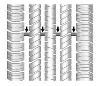
Treadwear indicators are one way to tell when it is time for new tires. Treadwear indicators appear when the tires have only 1.6 mm (1/16 in) or less of tread remaining. See *Tire Inspection on page 10-46* and *Tire Rotation on page 10-46*.
