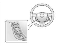
(On/Off): Press to turn the cruise control system on and off. A white cruise control indicator light turns on when in use.
