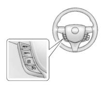
Press to turn the cruise control system on and off. A white cruise control indicator light turns on when in use.
