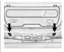
The top tether anchors are on the rear wall of the cargo area. Be sure to use an anchor on the same side of the vehicle as the seating position where the child restraint will be placed.
