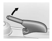
To set the parking brake, hold the brake pedal down and pull up on the parking brake lever. If the ignition is on, the brake system warning light will come on. See *Brake System Warning Light on page 5-14*.
