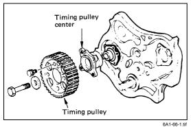
Remove the center bolt and remove the timing pulley with pulley center.
