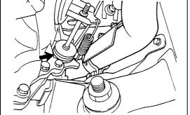
Remove the slave cylinder assembly with the flexible hose attached, and then tie it to the frame so that it does not interface with servicing work.
