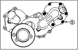
3) Temporarily tighten the six injection pump nuts ⑤. The injection pump nuts will be finally tightened after the injection pump rear bracket bolts.
