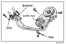
6. Power Steering Pump & Bracket Assembly (P/S Model)
