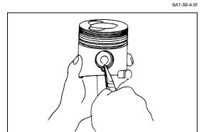
5) Use a pair of pliers to remove the piston pin snap rings.
