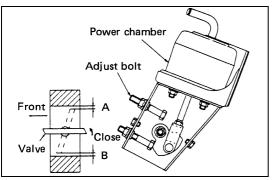
When the clearance is outside this range, adjust the clearance with the adjust bolt.
