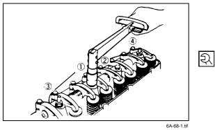
③ Tighten the rocker arm shaft bracket bolts to the specified torque in the numerical order shown in the illustration.
