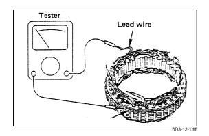
2. Check for continuity across one of the stator coils and stator core. If a continuity exists, replace the coil.
