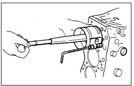
14) Position the piston head from mark so that it is facing the front of engine.
