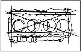
5. Use a straight edge ① and a feeler gauge ② to measure the four sides and the two diagonals of the cylinder body upper face.
