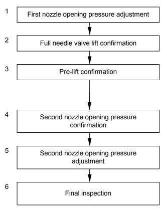
Adjust the first nozzle opening pressure using the shim.
