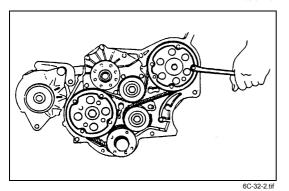
10. Flange; Camshaft Pulley
