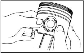
6) Use your fingers to force the piston pin snap ring into the piston snap ring groove.
