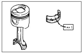
If the connecting rod upper bearings are to be reinstalled, mark their fitting positions by tagging each bearing with the cylinder number from which it was removed.
