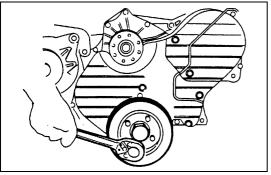
7. Crankshaft Dumper Pulley
