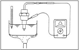
Use a circuit tester to check the thermo switch for continuity.
