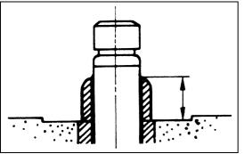
2. Apply engine oil to the outside of the valve guide. Using special tool, drive in a new valve guide from cylinder head upper face side, and check the valve guide height.
