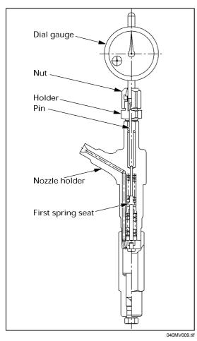
Secure the dial gauge to the nozzle holder using the nut so that the pin contacts the tip of the first spring seat.
