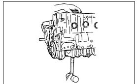
2) Move the piston to the top of the cylinder and tap it with a hammer grip or similar object from the connecting rod lower side to drive it out.
