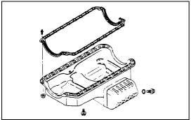
Remove the stiffener and space rubber from oil pan both side.
