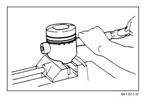
6) Tap the piston pin out with a hammer and a brass bar. If the pistons and piston pins are to be reinstalled, mark their installation positions by tagging each piston and piston pin with the cylinder number from which it was removed.
