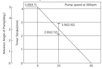
Temperature of wax element ( C) Indication timer stroke in parentheses.(mm) The timer stroke 1mm=1.22 on camshaft. The timer stroke 1mm=2.44 on crankshaft.
