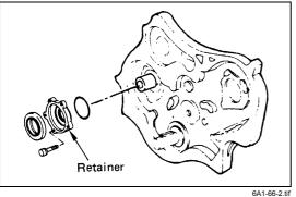
Remove the oil seal retainer.
