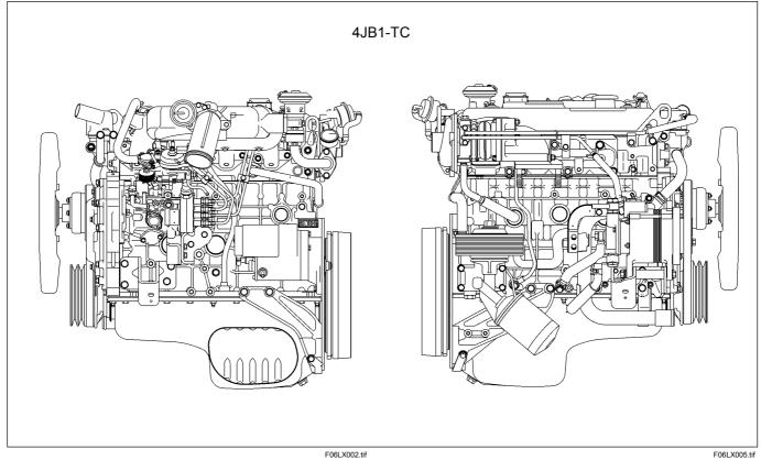
The 4JB1 Model engine employs a square troidal type combustion chamber provided with a fence around it. These designs employed allow a superior fuel economy over a wide range of driving conditions.
