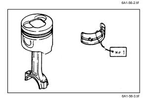
3) If the connecting rod upper bearings are to be reinstalled, mark their fitting positions by tagging each bearing with the cylinder number from which it was removed.
