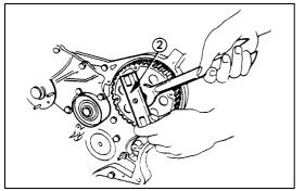
Use the timing pulley puller ② to remove the injection pump timing pulley.
