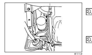
2. Front exhaust pipe mounting bracket fixing bolt and nut.
