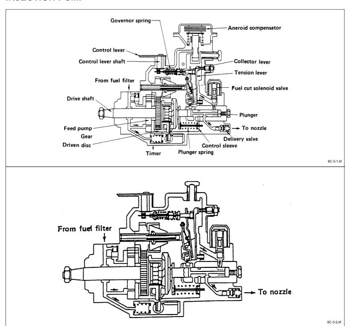
A Bosch Distributor Type Injection Pump is used. A single reciprocating/revolving plunger delivers the fuel uniformly to the injection nozzles, regardless of the number of cylinders.
