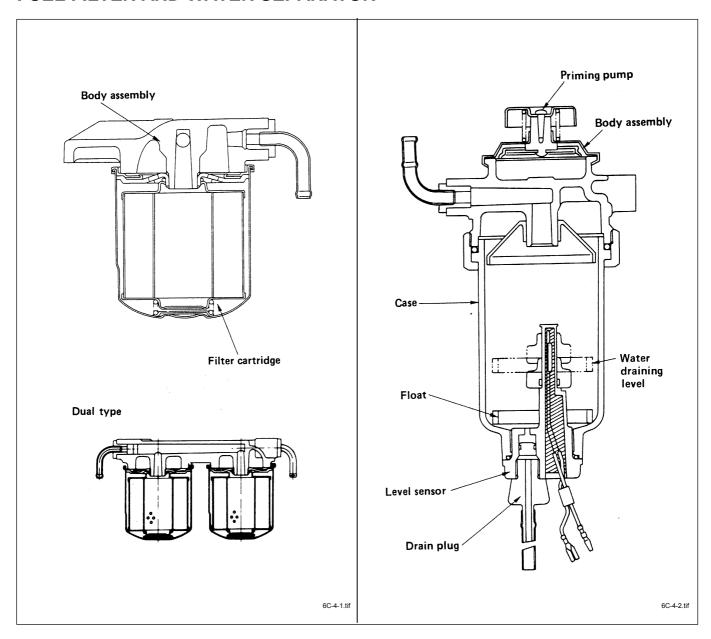
A cartridge type fuel filter and a water separator are used along with the VE type injection pump.
