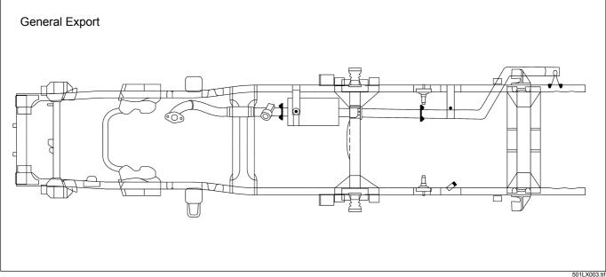
When inspecting or replacing exhaust system components, make sure there is adequate clearance from all points on the underbody to prevent overheating of the floor pan and possible damage to the passenger compartment insulation and trim materials.
