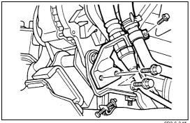
Install the suction pipe clip bolt and tighten bolt to the specified torque.
