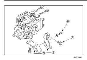
4) Install the injection pump rear bracket ⑥ and the rear bracket bolts ⑦ to the cylinder body.
