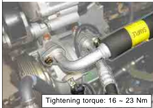
A/C Compressor Connector and Inlet/Outlet Pipes
