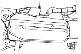
5. Remove the fuel tank. Remove the fuel gauge unit if necessary.
