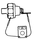
2. Insert a thin rod in the oil hole of the switch and push it in lightly. The switch is normal if no continuity is detected (infinite resistance on the tester). If there is continuity, replace the switch.
