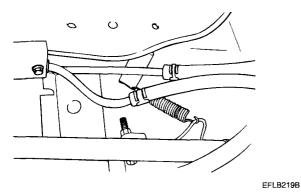
3. Disconnect the fuel gauge unit connector.
