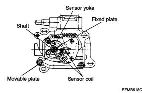
The control sleeve position sensor converts differences in the inductances of the upper and lower coils into angles, and feeds this back to the control unit. The control unit compares the target angle with the actual angle measured, and compensates the current so that the angle corresponds to the target angle.
