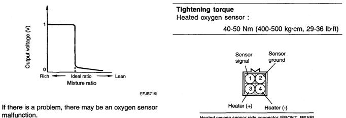
Heated oxygen sensor side connector (FRONT, REAR)
