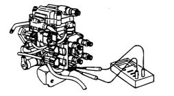
3. Confirm that there is continuity between the GE actuator connector terminal no 2 and no 10.
