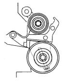
2. Install tensioner arm, shaft and plane washer to cylinder block.
