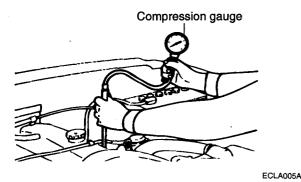
7. Crank the engine with the throttle valve fully open, and measure the compression at the place where the compression gauge indicator shows a stabilized reading.
