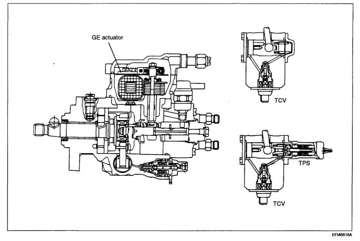
Refer to the VE type injection pump service manual for conventional injection pump construction and parts with common construction.
