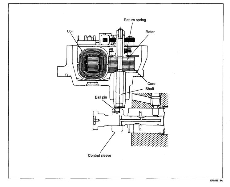
Unlike the conventional injection pump, COVEC-F adjusts fuel injection quantity electromagnetically. Control sleeve position is detected by the control sleeve position sensor and fed back to the control unit.
