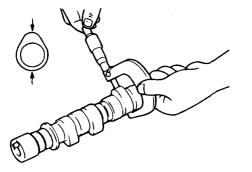
Check cam surfaces for abnormal wear and damage.
