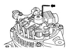
3. When installing a new brush, insert the brush into the holder, and then solder the lead wire.
