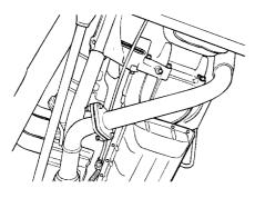
3. Remove the front exhaust pipe from the rubber hanger.
