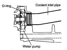
2. Install the new engine coolant pump gasket and pump assembly. Tighten the bolts to the specified torque.
