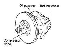
5. Check if there are foreign materials disturbing the oil flow in the oil passage of cartridge assembly.
