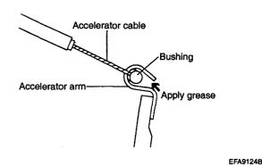
3. Securely install the resin bushing of the accelerator cable on the end of the accelerator arm.
