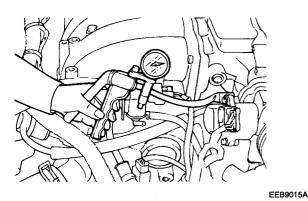
2. Start the engine and check to see that, after increasing the engine speed, vacuum rises fairly constantly.
