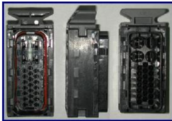
25-Pin Connector Used in MGH-25 ABS (P/No: AMP 368482-1)
