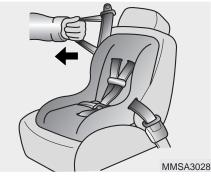
3. Pull the shoulder portion of the safety belt all the way out. When the shoulder portion of the safety belt is fully extended, it will shift the retractor to the "Auto Lock" (child restraint) mode.
