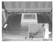
To keep items from shifting in the cargo area, you can use the four rings located in the cargo area to attach the luggage net.
