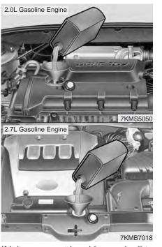
If it is near or at L, add enough oil to bring the level to F. **Do not overfill.**
