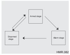
This system is designed to provide protection from unauthorized entry into the car. This system is operated in three stages: the first is the "Armed" stage, the second is the "Alarm" stage, and the third is the "Disarmed" stage. If triggered, the system provides an audible alarm with blinking of the hazard warning lights.
