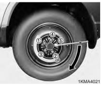
11. Once the wheel lug nuts have been tightened, lower the vehicle fully to the ground and continue to tighten the lug nuts until they are fully secured. Tighten the wheel lug nuts firmly in a "star" pattern.
