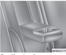
*Rear (if equipped)* To use the cup holders in rear seat, pull down the rear seat armrest.
