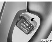
3. Push down the - / SET switch, and release it at the speed you want. The "SET" indicator light in the instrument cluster will illuminate. Release the accelerator at the same time. The desired speed will automatically be maintained.
