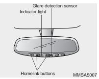
Your new mirror comes with an integrated HomeLink Universal Transceiver, which allows you to program the mirror to activate your garage door(s), estate gate, home lighting, etc. The mirror actually learns the codes from your various existing transmitters.
