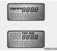
TRIP A: Tripmeter A TRIP B: Tripmeter B
