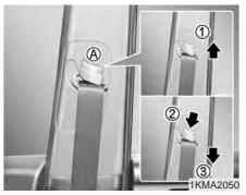
Adjust the shoulder anchor position to your size. To raise the anchor position, push the anchor up (①). To lower the anchor position, press (②) the button (A) and slide the anchor down (③). After adjustment, make sure the anchor is locked in position.
