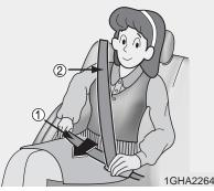
4. Position the lap portion (①) of the belt across your lap as LOW ON THE HIPS as possible to reduce the risk of sliding under it during an accident. Adjust the belt to a SNUG FIT by pulling up on the shoulder portion (②) of the safety belt. The belt retractor is designed to take up excess webbing automatically and to maintain tension on the belt. For your safety do not put any excess slack into the safety belt.
