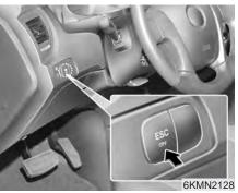
The Electronic Stability Control (ESC) monitors information from various vehicle sensors and then compares the driver's commands with the actual behavior of the vehicle.
