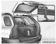
2. Detach the hook from the cover and hang the hook on the weather strip.
