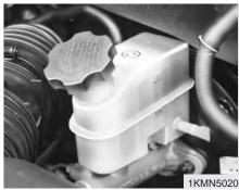
If the level is low, add fluid to the MAX level. The level will fall with accumulated mileage. This is a normal condition associated with the wear of the brake linings. If the fluid level is excessively low, have the brake system checked by an Authorized Kia Dealer.
