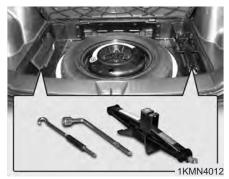
The spare tire, jack, jack handle, wheel lug nut wrench are stored in the luggage compartment. Remove the luggage under tray out of the way to reach this equipment.
