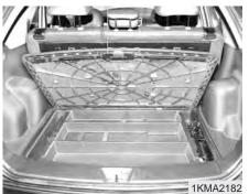
The luggage center box is located under the floor in cargo area. You can place a first aid kit, a reflector triangle, tools, etc. in the box for easy access.
