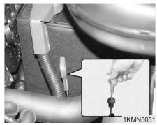
Checking the automatic transaxle fluid level
