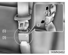
2. To retract the rear center seatbelt, insert the key or similar small rigid device into the web release button on the anchor connector. Pull up on the seat belt web (A) and allow the webbing to retract automatically.
