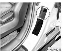
All specifications (sizes and pressures) can be found on a label attached to the front driver's door sill.
