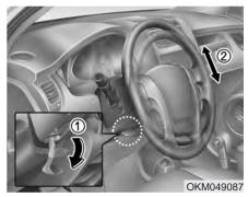
To change the steering wheel angle, pull down (①) the lock release lever, adjust the steering wheel to the desired angle (@), then pull up the lock-release lever to lock the steering wheel in place.
