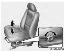
Adjusting the height of seat cushion (for driver's seat, if equipped) To change the height of the seat cushion, rotate the knob located on the outside of the seat cushion.
