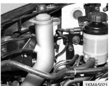
Checking the washer fluid level
