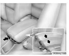
To use the center console as armrest (if equipped), push the release button then it rises.
