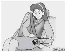
3. Insert the tongue plate (①) into the open end of the buckle (②) until an audible "click" is heard, indicating the belt is locked in the buckle.
