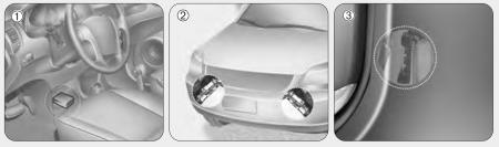
Airbag collision sensors① SRS control module
