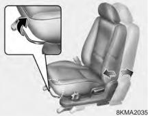
Adjust the seat before driving, and make sure the seat is locked securely by trying to move forward and backward without using the control knob. If the seat moves, it is not locked properly.
