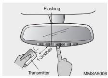
2. Press and hold the button on the HomeLink system you wish to train and the button on the transmitter while the transmitter is approximately 1 to 3 inches away from the mirror. Do not release the buttons until step 3 has been completed. 3. The HomeLink indicator light will flash, first slowly and then rapidly. When the indicator light flashes rapidly, both buttons may be released. (The rapid flashing light indicates successful programming of the new frequency signal.)
