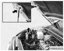
3. Lift the hood and hold it open with the support rod by inserting the free end of the rod into the slot (①).
