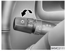
**Parklight position ( EVEC )** When the light switch is in the parklight position (1st position), the tail, position, license and instrument panel lights are ON.
