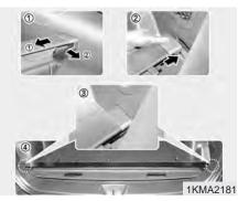
When not in use, place the tonneau cover on the lower portion of cargo area.
