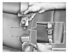
2. Insert the tongue plate (A) into the open end of the buckle (C) until an audible "click" is heard, indicating the latch is locked. Make sure the belt is not twisted.
