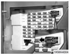
5. Push in a new fuse of the same rating, and make sure it fits tightly in the clips.
