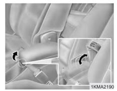
*Type B (if equipped)* To open the console storage compartment, pull up on the locking tab.
