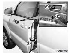
To lock a door without the key, push the inside door lock button (①) or door lock switch (②), if equipped) to the "Lock" position and close the door (③).
