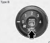
OKM049126 The defroster heats the window to remove frost, fog and thin ice from the interior and exterior of the rear window, while engine is running.
