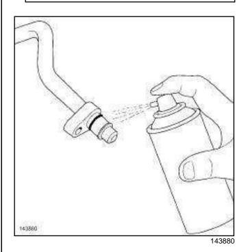
□ Clean the surface and seal of the pipe using EN-GINE CLEANER (see Vehicle: Parts and consumables for the repair) (04B, Consumables -Products).
