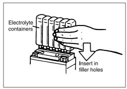
Make sure air bubbles are coming up each electrolyte container, and leave in this position for about more than 20 minutes.
