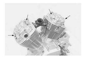
• Remove the front cylinder head cover.
