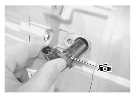
• Apply the THREAD LOCK to the speed sensor bolt and tighten it
