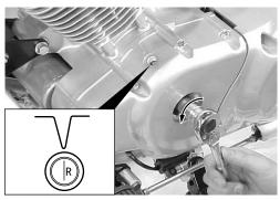
• To inspect the No.1 cylinder's valve clearance, insert the thickness gauge to the clearance between the valve stem end and the adjusting screw on the rocker arms.
