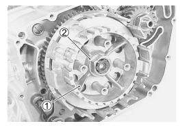
• Install the clutch sleeve hub nut, and tighten it to the specified torque using the special tool.
