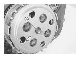
• Tighten the clutch cover bolts securely.
