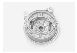
• Remove the rear brake cam lever ① and rear brake cam ② by removing nut.
