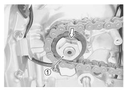
• Remove the engine sprocket.
