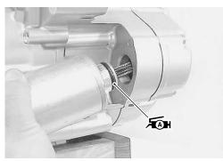
• Mount the starter motor on the engine.
