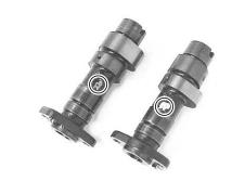
Apply MOLYBDENUM OIL to the camshaft journals and cam faces.
