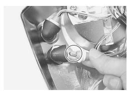
Remove the speedometer from speedometer cover by removing the screws.
