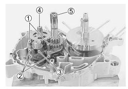
• Remove the crankshaft by using the special tool.
