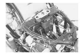
Disconnect the rear turn signal light couplers and rear combination light coupler.
