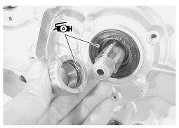
• Install the oil seal retainer.
