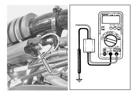
Inspect No. 2 ignition coil primary peak voltage in the same manner of No. 1 ignition coil inspection.
