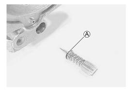
• Apply grease to the O-ring and install the accelerating plunger.
