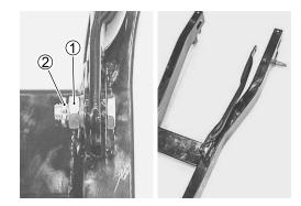
• Install the swingarm and tighten the swingarm pivot nut to the specified torque.
