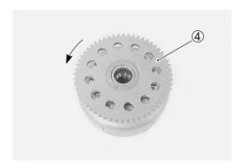
Install the rotor with the starter driven gear onto the crankshaft securely.
