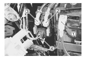
Apply 12 volts to A and B terminals, inspect the continuity between the terminals, positive and negative.
