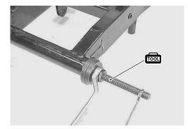
• Install the torque link and washer ①, tighten the torque link nut to the specified torque.
