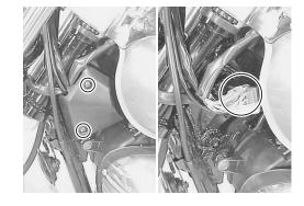
• Remove the fuel tank mounting nut and bolt.
