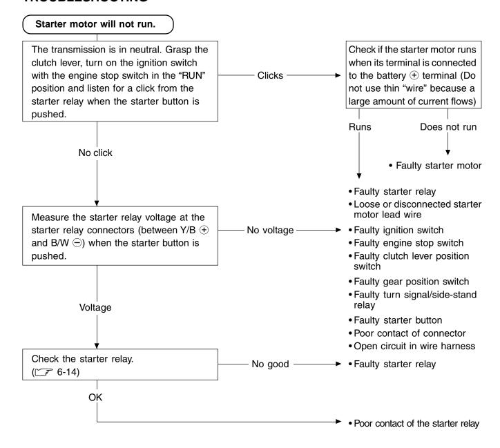
The starter motor runs when the transmission is in neutral, but does not run when the transmission is in any position other than neutral, with the side-stand up.
