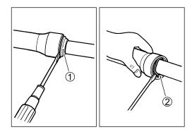
• Separate the inner tube from the outer tube.
