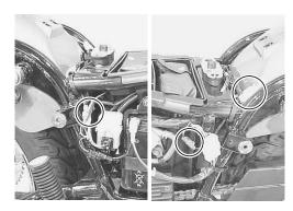
• With the bolt removed, remove the rear fender.
