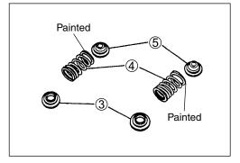
· Compress the valve spring using the valve lifter and the attachment.
