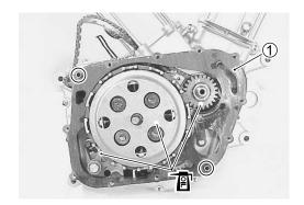
• Face the rack teeth (A) backward and align the clutch release rack with the pinion gear.
