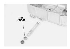
• Drive in the oil seal using the special tool.
