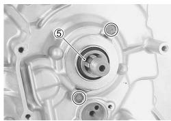
• Remove the crankcase securing bolts.
