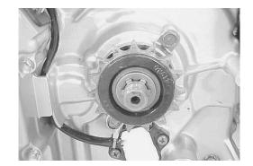
• Tighten the engine sprocket nut 1 to the specified torque.
