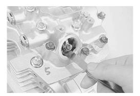
Apply grease to the new O-ring and install the valve inspection caps.
