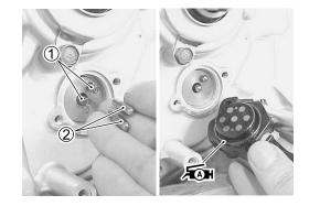
Pass through the gear position switch wire harness into the guide
