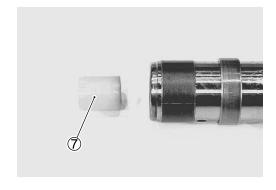
Apply grease to the lip of the oil seal ③ and install it into the outer tube using the front fork oil seal installer.
