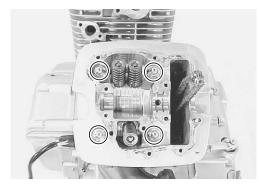
• Remove the gasket ①, cam chain guide ② and cylinder.
