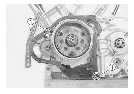
Install the generator cover and tighten the generator cover bolts.
