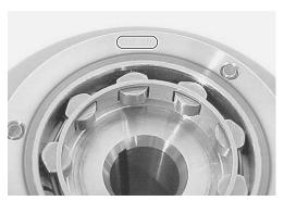
Apply a small quantity of THREAD LOCK SUPER "1303" to the starter clutch bolts and tighten them to the specified torque while holding the rotor holder.
