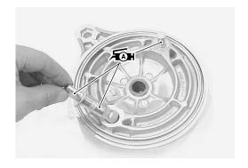
Install the brake shoes with spring hooks faced inside.
