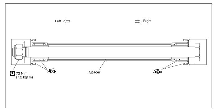
Press the needle bearings into the swingarm pivot using the special tool.
