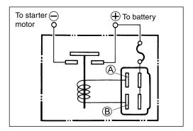
• Check the coil for "open", "ground" and ohmic resistance. The coil is in good condition if the resistance is as follows.
