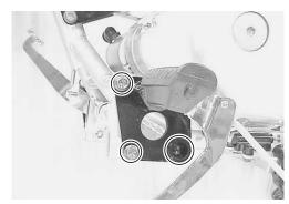
Install the gearshift arm and adjust the gearshift lever hight.
