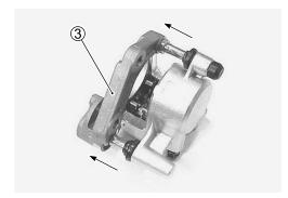
• Using an air blow gun, pressurize the caliper fluid chamber to push out the piston.
