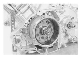
• With the generator rotor held immovable using special tool, tighten the generator rotor nut to the specified torque.
