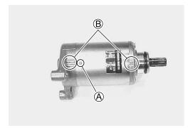
• Apply grease to the O-ring, and remount the starter motor.
