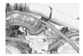
• With the bolts removed, take out the center air cleaner box.
