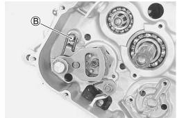
• Install the washer ® and circlip 9.
