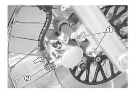
• Fill the system with brake fluid and bleed air. ( 2-14)
