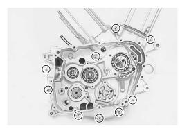
• Separate the crankcase into 2 parts, right and left, with a crankcase separating tool.
