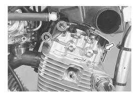
• Remove the generator cover plug 1) and the timing inspection plug 2.
