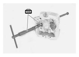
• Remove the valve cotter halves ①.
