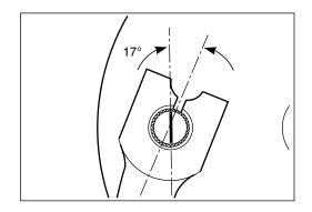
• Tighten the brake cam lever nut to the specified torque.
