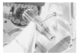
• Install the starter driven gear 4 to the starter clutch rotating the starter driven gear.
