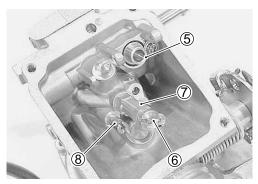
· Remove the throttle cable bracket.
