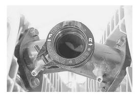
• Apply the THREAD LOCK to the bolts and tighten them.
