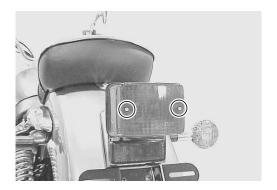
• Push in on the bulb ①, turn it counterclockwise, and pull it out.
