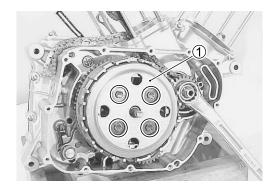
• Remove the clutch drive and driven plates.
