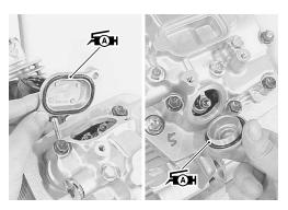
• Install the generator cover plug ① and timing inspection plug ②.
