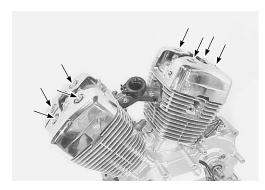
• Remove the valve inspection caps.
