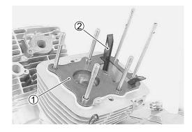
• Remove the No. 2 (Front) cylinder head and cylinder in same manner of No. 1 (Rear) cylinder head and cylinder removal.
