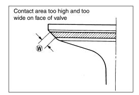
(Use the 32° cutter for intake.) (Use the 15° cutter for exhaust.)
