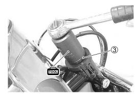
• Remove the handlebar holders by removing the nuts.
