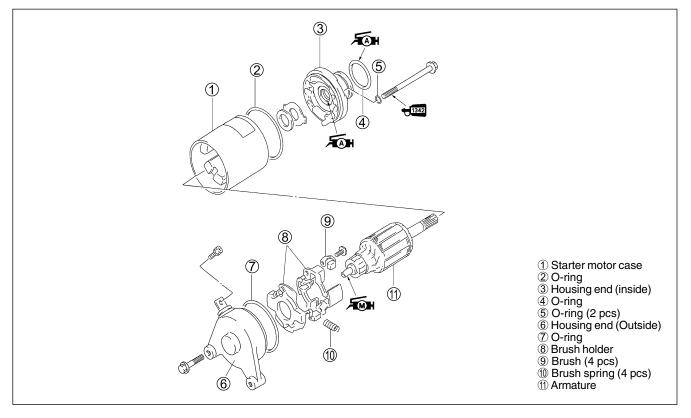
• Align the mark (A) on the housing with the line (B) on the housing end.
