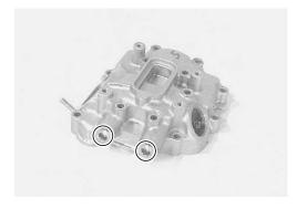
• Draw out the rocker arm shaft ① using 6 mm bolt.
