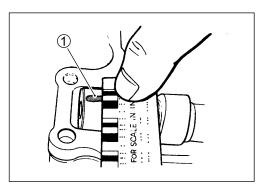
If the clearance exceeds the service limit, measure the inside diameter of camshaft journal holder using a cylinder gauge.
