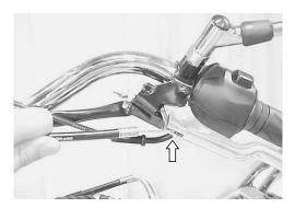
• Disconnect the clutch cable end out of clutch release arm.
