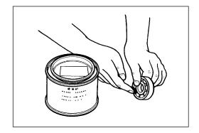
• Press fit the bearing to the wheel using the special tools.
