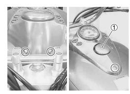
• Remove the bulb socket and pick up the indicator bulbs.
