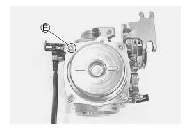
Apply thermo-grease to the threads and tighten the carburetor heater. (Only for E-02)
