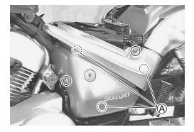
• With the seat lock cable disconnected, remove the left frame cover.
