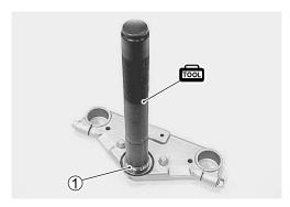
· Apply grease to the upper bearing, lower bearing and outer races prior to installing the steering stem.
