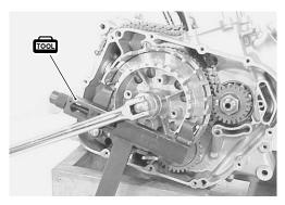
• Remove the clutch sleeve hub ③ and primary driven gear assembly ④.
