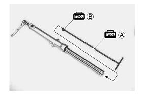
• Remove the damper rod ⑦ and rebound spring ® from the inner tube.
