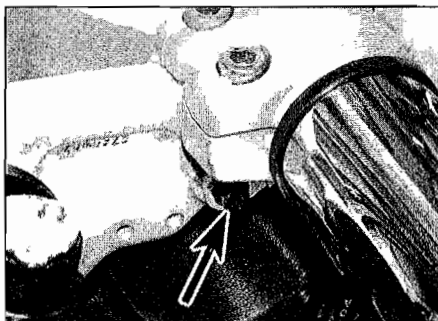
16.6c ... and unscrew the positioning bolt (arrowed)
