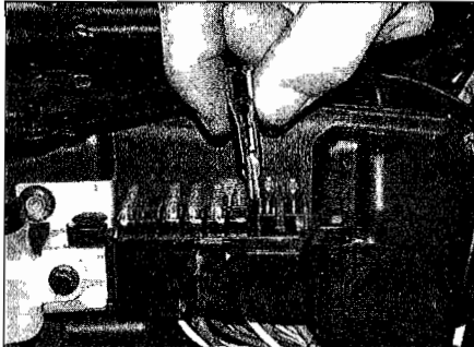
5.3a Use the tool provided to remove a fuse
