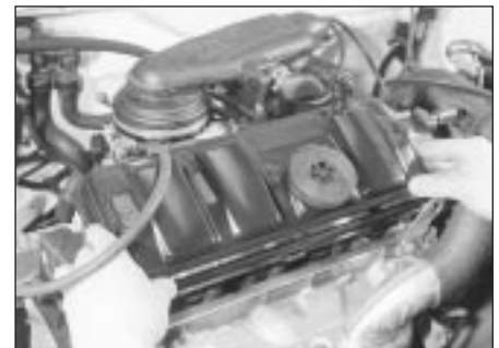
4.5 . . . and lift off the cylinder head cover
