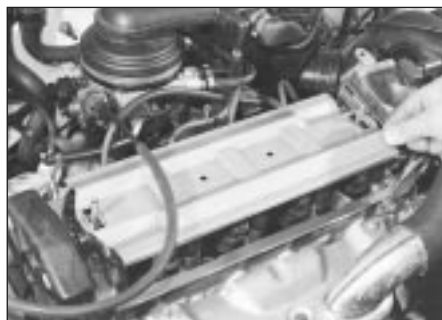
4.6b . . . and remove the oil baffle plate
