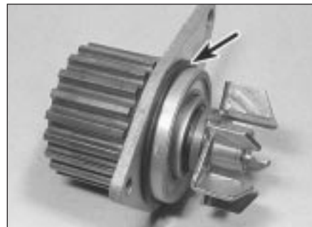
8.18b ... then recover the O-ring seal (arrowed)
