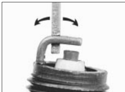
Adjusting spark plug gap
