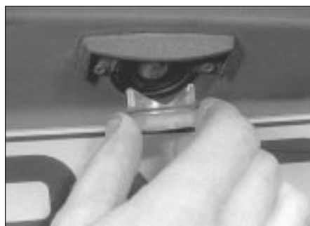
8.22 Remove the rear number plate light lens . . .
