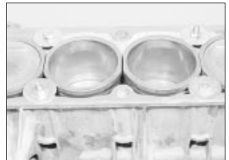
8.17 Cylinder liners clamped with washers and bolts
