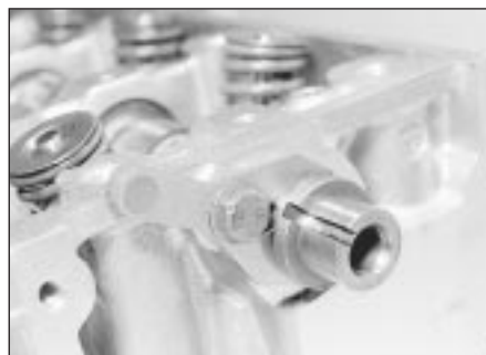
6.7 Camshaft retaining thrust plate
