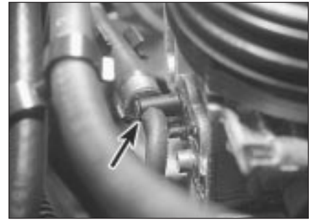
11.25 Vacuum hose connection to throttle body (arrowed)
