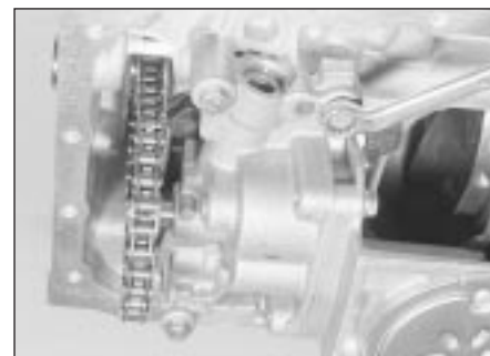
13.2 The oil pump is retained by three bolts
