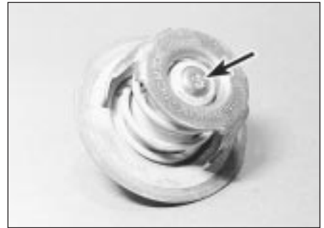
4.9 Thermostat temperature rating (arrowed) stamped on base
