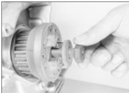
8.11a Remove the crankshaft sprocket bolt . . .
