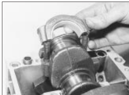
7.5 Remove the big-end bearing caps
