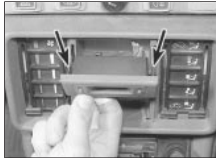
26.5 Digital clock and retaining barbs (arrowed)
