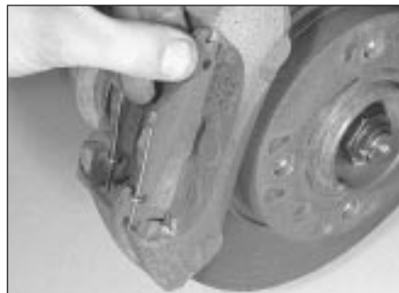
4.5 Removing the outer pad (DBA Bendix caliper)
