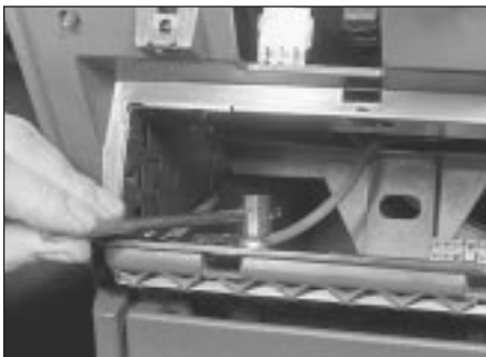
26.34a Removing the centre console upper nuts . . .
