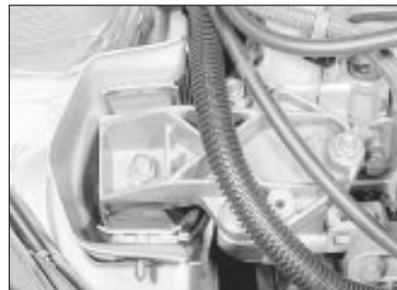
8.6 Right-hand engine mounting and cylinder head bracket
