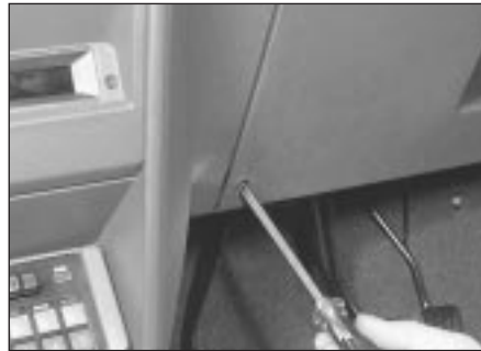
26.16 Removing a right-hand lower facia panel securing screw
