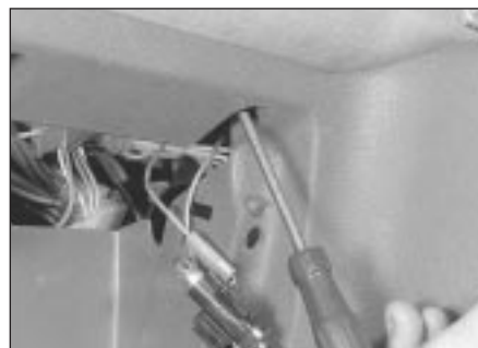
26.11 Removing a facia mounting screw
