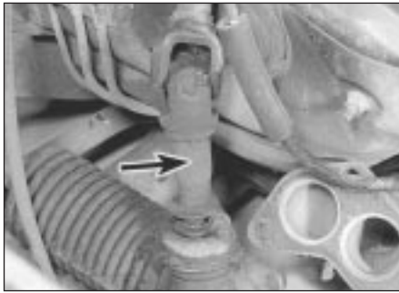
14.7 Steering column intermediate shaft (arrowed)
