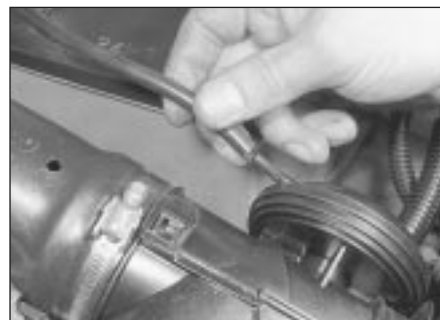
2.9 Disconnect the hose from the vacuum motor
