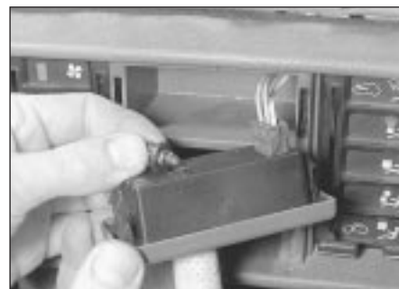
9.11 Removing digital clock illumination light bulb
