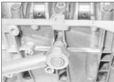
13.60 Refit and tighten the centre main bearing side bolts
