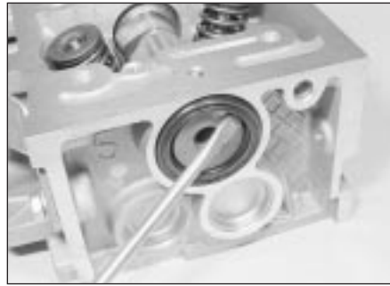
10.9a . . . prise out the oil seal . . .
