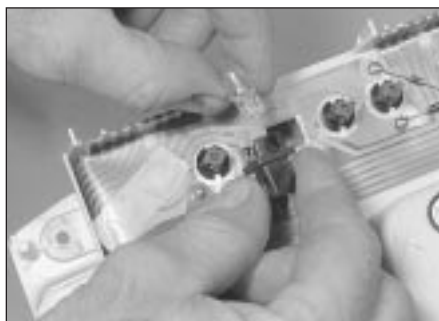
9.7 Removing square type instrument panel bulbholder
