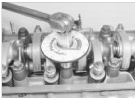
11.38 ... then with an angle tightening gauge
