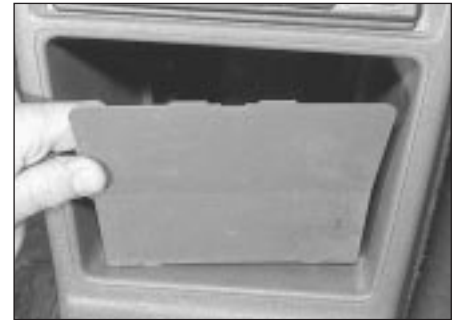
26.6 Removing the rear of the oddments tray
