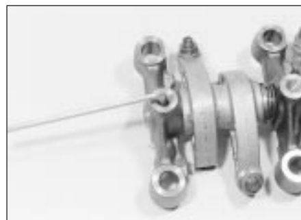
10.5b . . . then remove the grub screw
