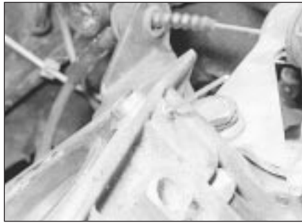
7.39 Using a pop rivet to retain the cylinder head location dowel
