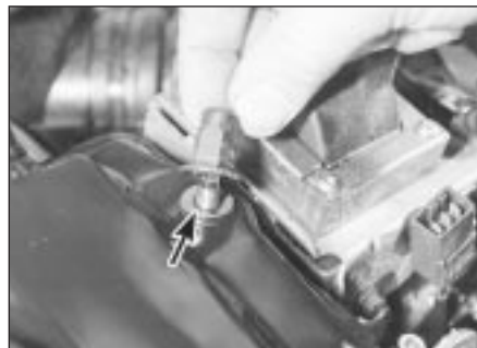
4.4 . . . then slacken and remove the cover retaining nuts and washers (arrowed) . . .
