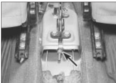
15.5 Handbrake adjustment nut and locknut (arrowed)
