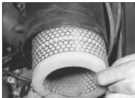
26.2 . . . and remove the cover and filter element
