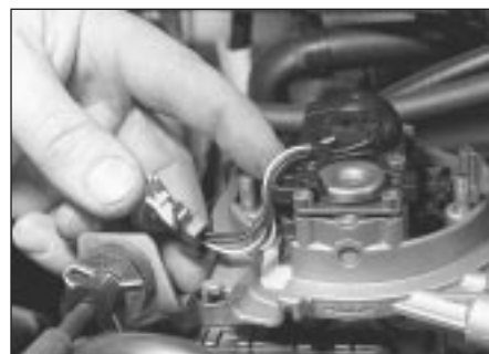
11.12b . . . then release wiring from clip
