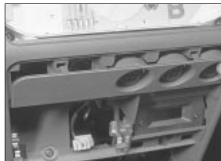
4.13c . . . and withdraw the switch panel surround
