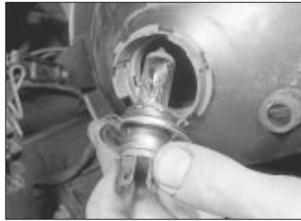
8.7b ... and withdraw the headlight bulb
