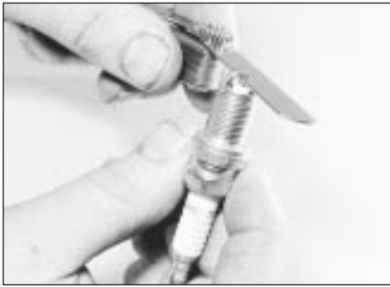
7.9 Measuring the spark plug gap with a feeler blade
