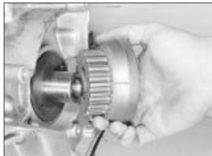
8.11b . . . then slide off the sprocket
