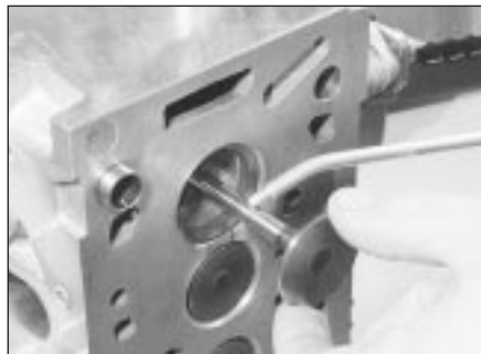
6.27 Lubricate the valve stems prior to refitting
