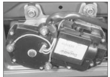
16.6 Tailgate wiper motor and mounting bolts
