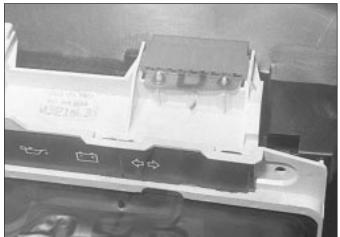
5.6b Instrument panel right-hand upper multiplug
