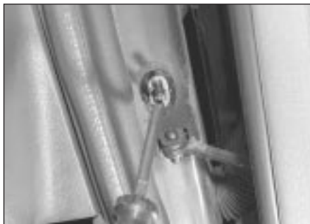
4.21 Removing a courtesy light switch
