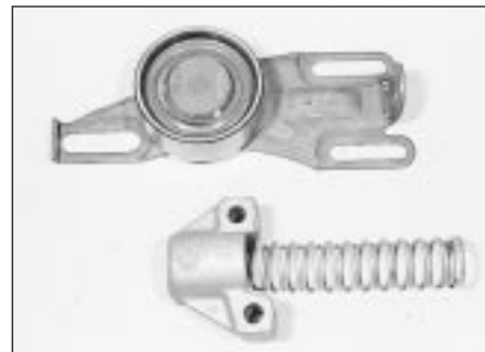
5.12 Spring loaded timing belt tensioner components
