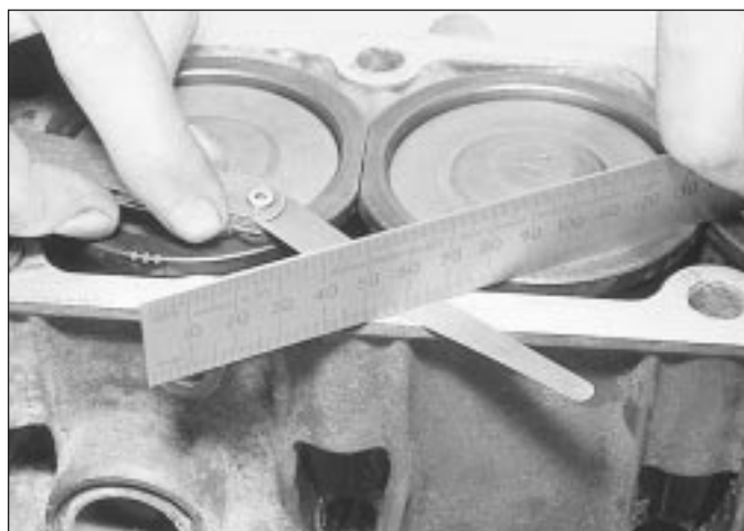
9.24 Measuring cylinder liner protrusion
