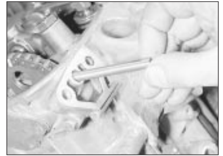
7.21 Removing the fuel pump plunger
