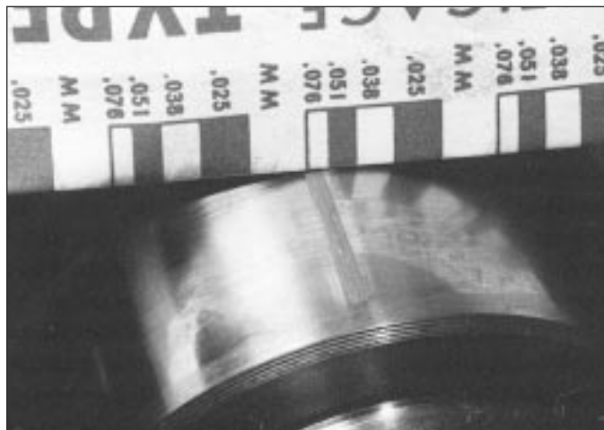
13.29 Measure the width of the deformed Plastigage using the scale on the card
