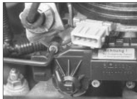
11.16 Unscrewing an idle speed control motor securing screw
