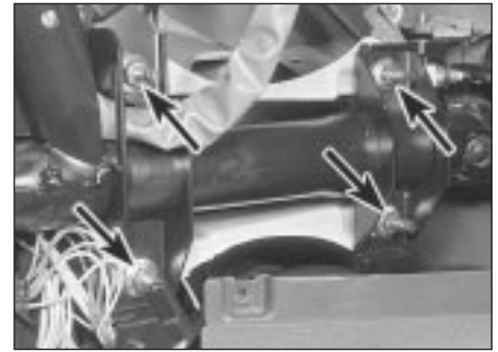
26.29 Steering column mounting nuts (arrowed)
