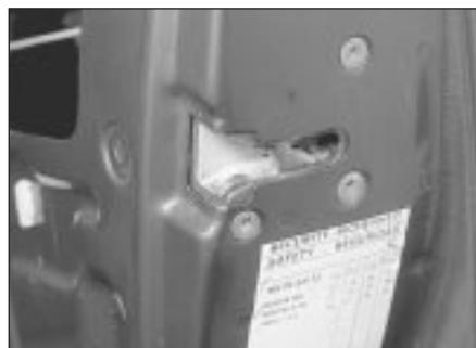
12.3a Door lock and mounting screws
