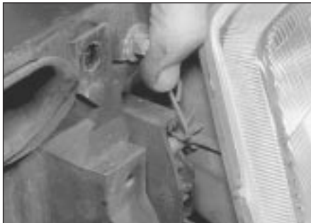
10.3 Releasing the headlight spring clips
