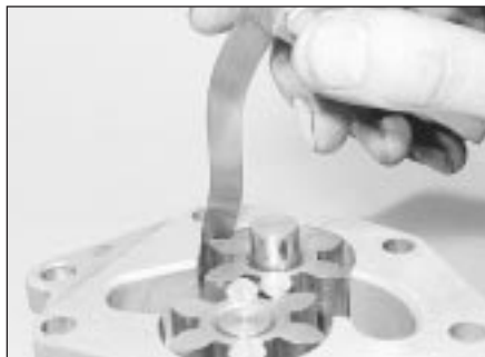
5.6 Checking oil pump gear to body clearance
