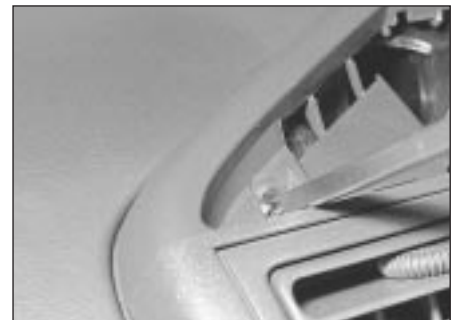
26.22a Removing the central vent assembly upper . . .
