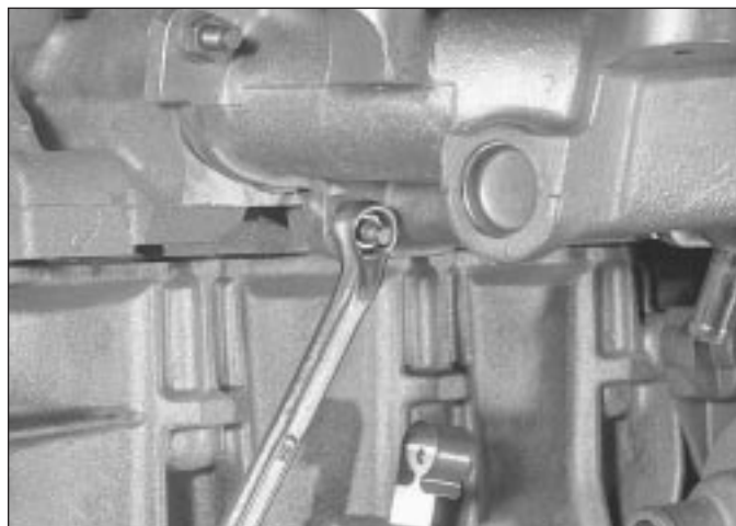
11.6 Unscrewing the inlet manifold retaining nuts - TU series engine shown
