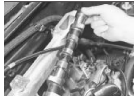
7.9 Lift the camshaft from the cylinder head
