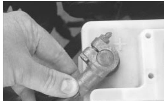
D Check the security and condition of the battery terminals.
