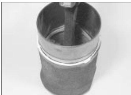
9.11 Cylinder liner with paper base seal
