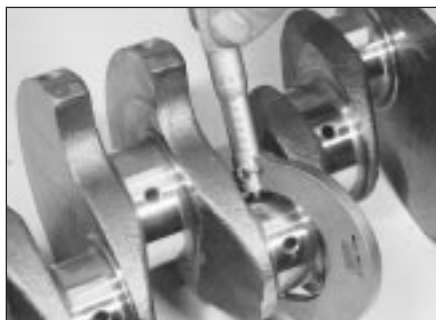
8.40 Measuring a crankshaft big-end journal diameter
