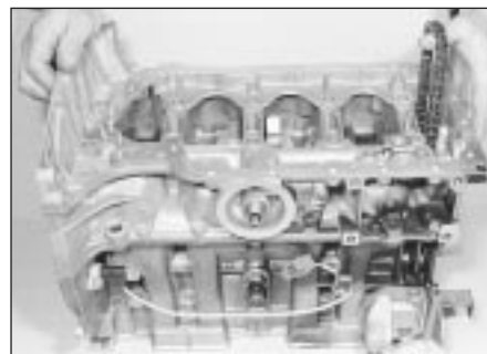
13.74 . . . then lower the main bearing ladder into position
