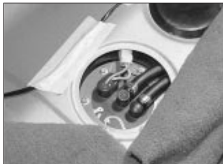
5.3 Fuel pump locations and connections
