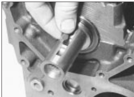
8.12b . . . and remove the Woodruff key
