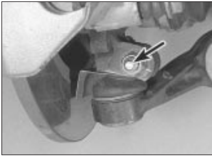
2.4a Unscrew the lower balljoint clamp bolt . . .
