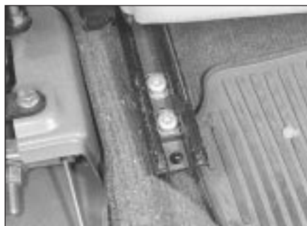
21.1 Front seat rear inner mounting bolts
