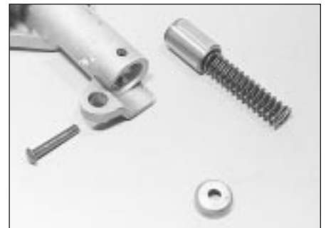
5.8 Oil pump pressure relief valve components
