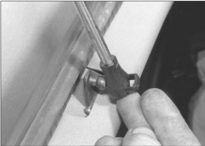
16.2 Disconnecting the tailgate struts
