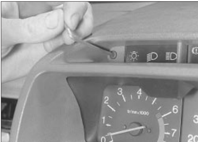
5.2 Removing the instrument panel upper ...
