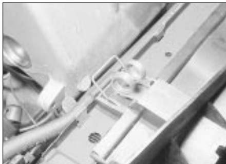
6.1a Radiator cooling fan retaining clip
