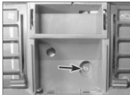
26.9 Facia mounting screw located in the ashtray recess (arrowed)
