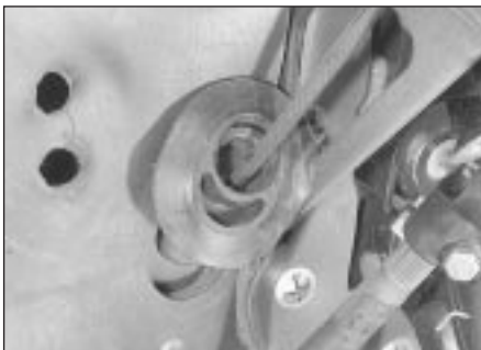
7.3b Speedometer cable grommet on the bulkhead
