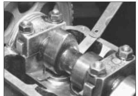
12.8 Checking a valve clearance - 1.6 and 1.8 litre
