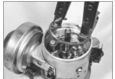
7.10b Removing bearing plate retaining ring
