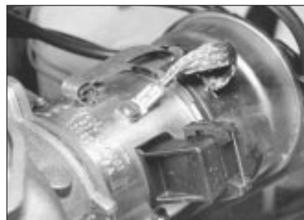
11.10 Fitting distributor cap and earth lead
