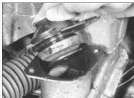
8.1a Lift the mounting away
