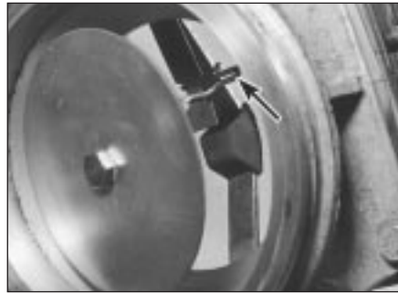
14.6 Airflow sensor plate adjustment clip (arrowed)
