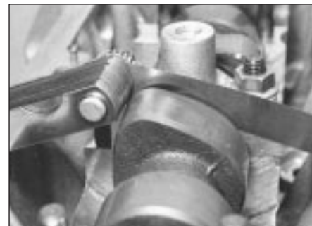
8.6 Measuring camshaft endfloat
