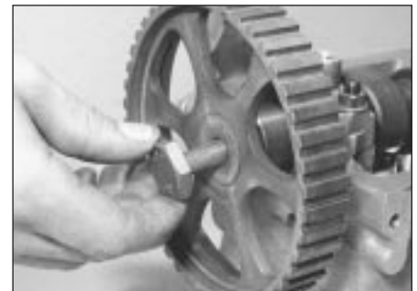
10.8 Fitting the camshaft sprocket bolt
