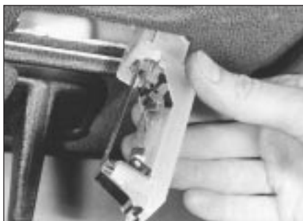
8.13b Interior light removal – 1.8 litre
