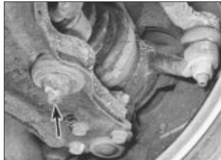
4.2 Anti-roll bar eye bolt nut (arrowed)
