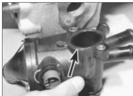
11.4 O-ring (arrowed) in thermostat housing
