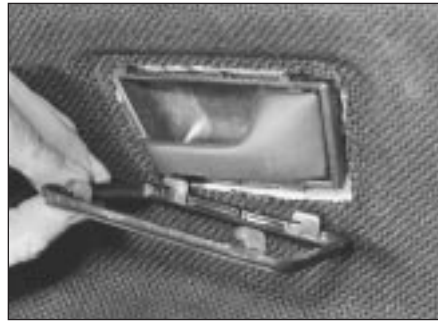
14.2 Removing door inner handle surround
