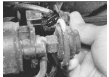
19.4 Disconnecting wiring connector from fuel pump
