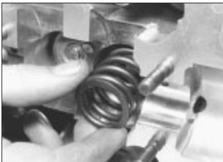
5.11a Removing an outer valve spring
