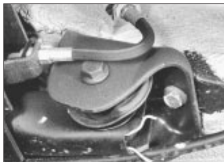
9.7 Axle beam pivot bolt head fitting position
