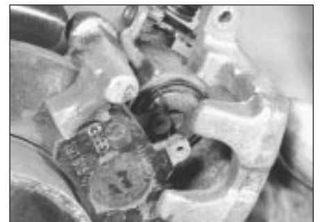
2.17 Rear brake caliper removal
