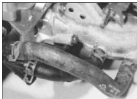
11.5 Coolant hoses in position
