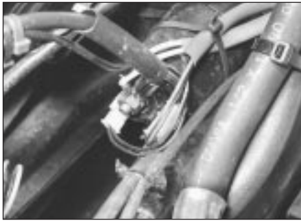
10.4 Starting motor solenoid wiring connections – 1.3 litre
