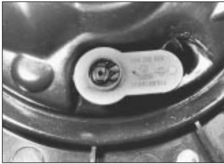
4.5 Upper view of air temperature sensor - 1.3 litre
