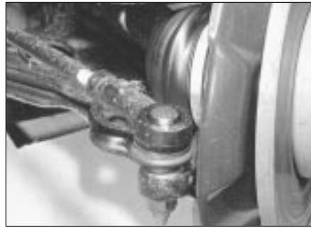
15.1 Right-hand adjustable balljoint
