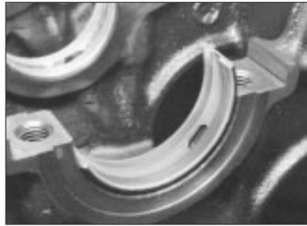
30.3b Fitting alternative type centre main bearing into crankcase . . .
