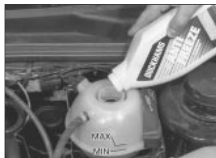
2.13 Topping-up engine coolant
