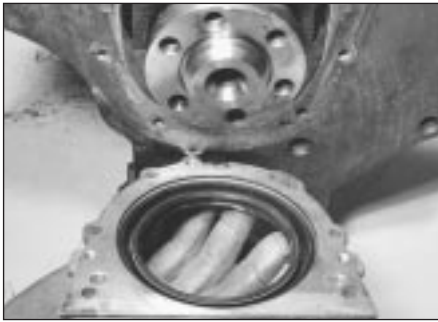
14.13a Withdrawing crankshaft rear oil seal housing . . .
