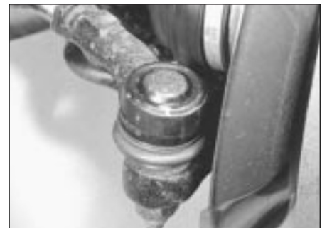
28.2 Inspect balljoint dust covers
