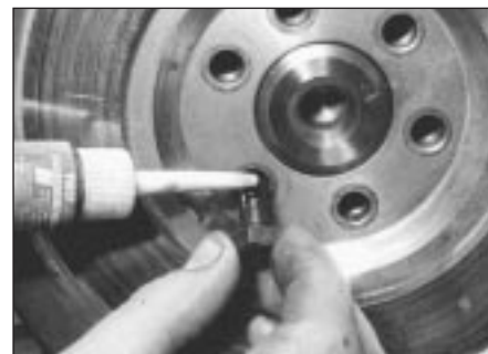
33.3 Applying liquid locking fluid to flywheel bolts
