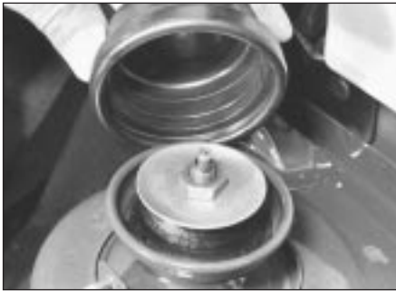
8.4 Removing rear suspension strut top cap
