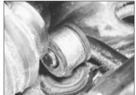
4.5 Anti-roll bar location in eye bolt
