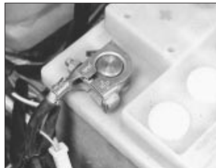
4.2 Battery positive terminal connection
