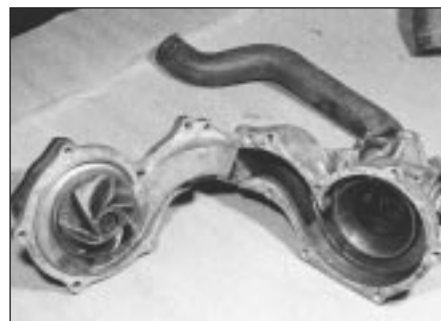
6.17 Two halves of coolant pump - 1.6 and 1.8 litre
