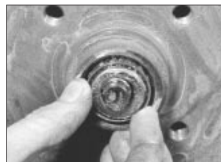
6.5c ... and outer bearing
