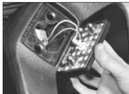
11.3a Removing steering wheel centre cover - 1.3 litre
