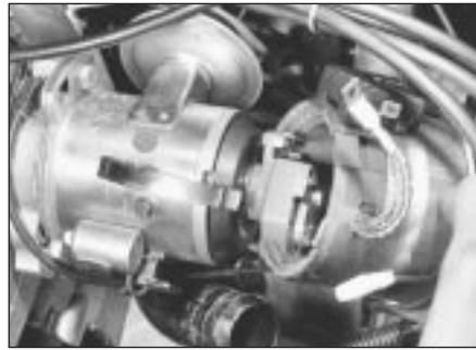
11.2 Withdraw distributor cap and screen ring
