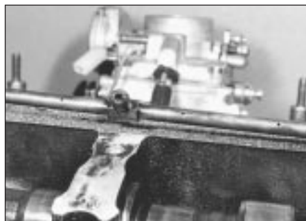
10.7 Removing oil spray tube
