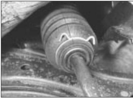
14.4 Steering tie-rod bellows and retaining clip
