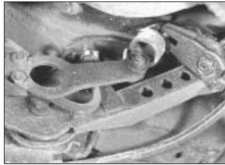
10.1 Brake pressure regulator unit
