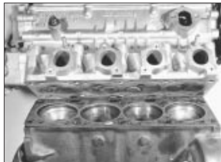
9.9 Removing cylinder head . . .
