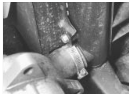
2.4b Radiator bottom hose connection - 1.8 litre
