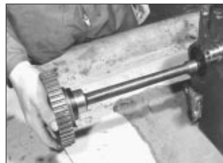
16.5b Withdrawing intermediate shaft
