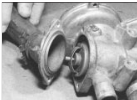
5.11b . . . withdraw thermostat elbow . . .
