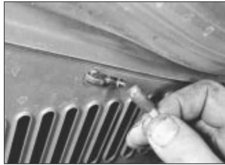
6.3 Disconnecting windscreen washer tubes from bonnet
