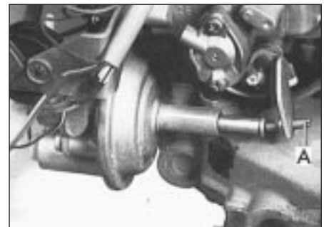
17.39b Fast idle adjustment screw (A)
