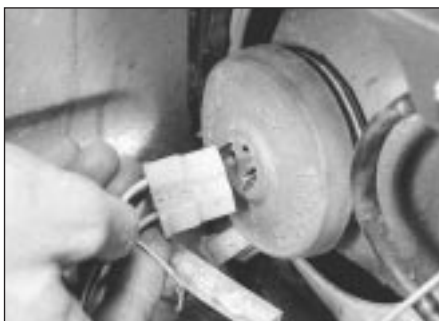
4.1 Detaching headlamp bulb connector
