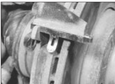
2.9 Pad retaining spring is located as shown
