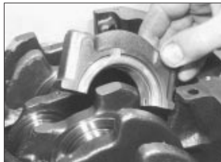
30.5 Fitting main bearing caps
