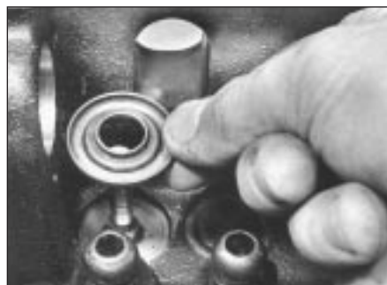
11.4 . . . and valve spring lower seats
