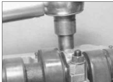
10.5 Tightening a camshaft bearing cap nut
