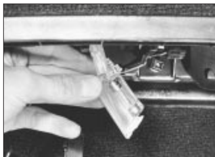
8.16 Luggage compartment lamp lens removal
