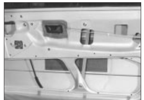
14.10 Plastic cover peeled back for access to door components
