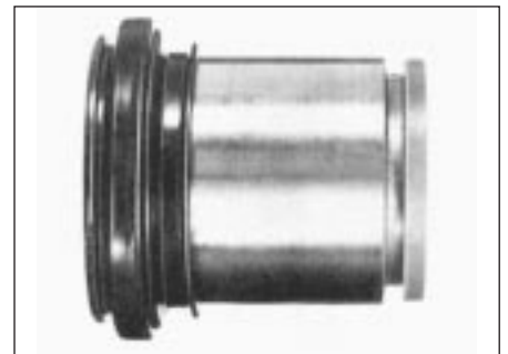
3.9 Dust seal location on caliper piston
