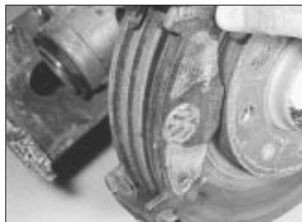
2.10 Refitting front brake pads
