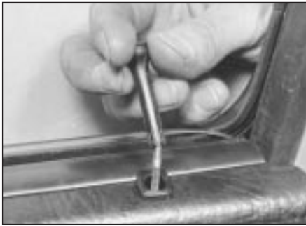
14.1 Unscrewing door locking knob
