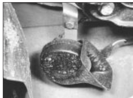
24.1b High tone horn location - twin horn installation
