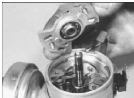
16.3 Removing the bearing plate - 1.05 and 1.3 litre
