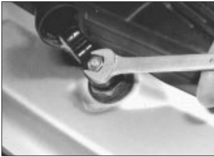
26.2 Undo wiper arm nut . . .
