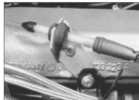
8.10 Accelerator cable adjuster and support bracket
