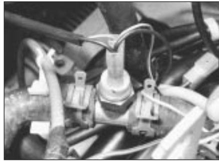
7.11 Temperature sender unit thermo-switch location - 1.05 and 1.3 litre
