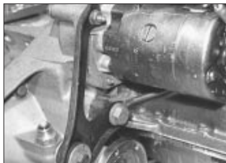
6.3 Starter motor and exhaust support bracket
