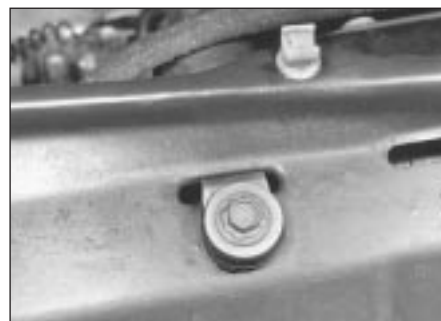
3.5 Radiator central retaining bolt and bracket
