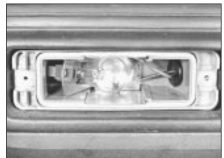
8.5 Front indicator lamp bulb
