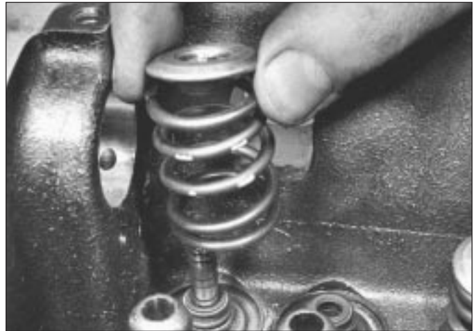
11.2b Removing valve springs and retainers . . .
