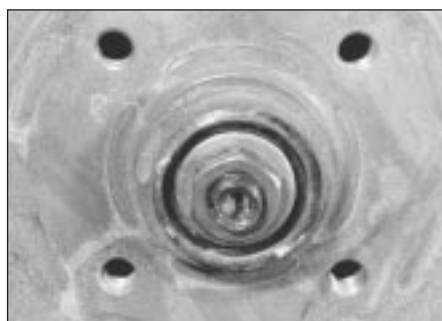
6.5a Undo the hub nut ...
