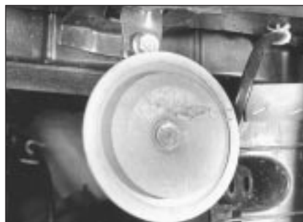
24.1a Single horn location behind front grille
