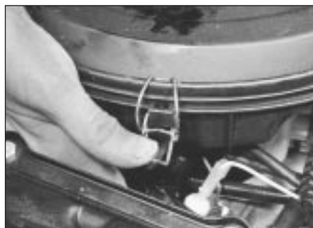
32.1 Unclip the air cleaner lid . . .
