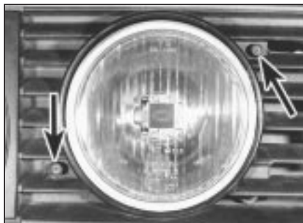
7.4 Foglight beam alignment adjuster screws (arrowed)
