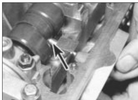
11.6 Fitting fuel pump plunger (arrowed)
