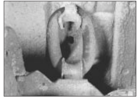
19.3 Check exhaust system mountings
