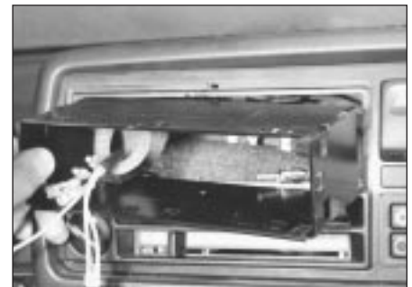
31.6 Radio/cassette container removal
