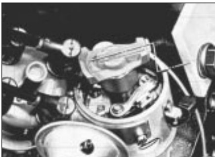
7.6b Rotor arm aligned with TDC mark on distributor body
