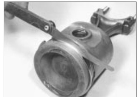
23.7b Checking piston ring-to-groove wall clearance
