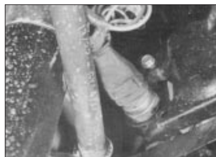
3.3a Radiator thermo-switch - 1.8 litre
