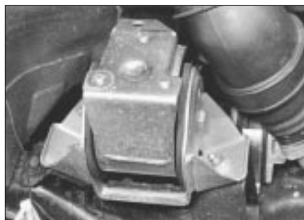
8.1b Right-hand rear mounting viewed from above
