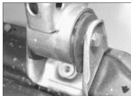
5.25a Engine/gearbox unit front mounting
