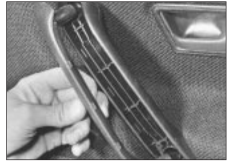
14.3a Removing door pull cover
