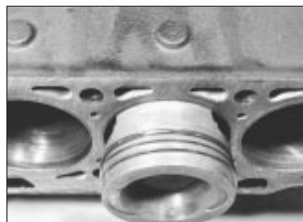
17.8 Removing a piston
