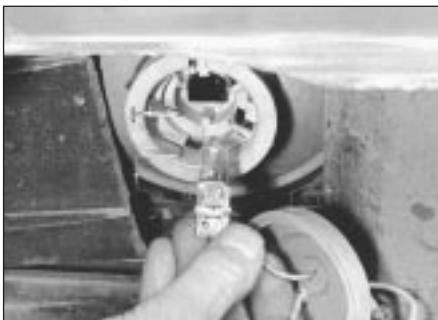
7.2 Bulb and holder removal from foglight
