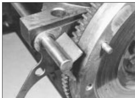
13.2 One method of holding the flywheel stationary
