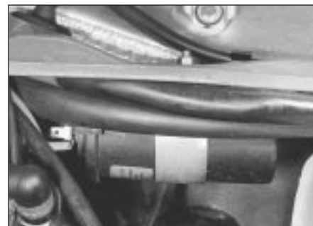
9.1 Ignition coil location
