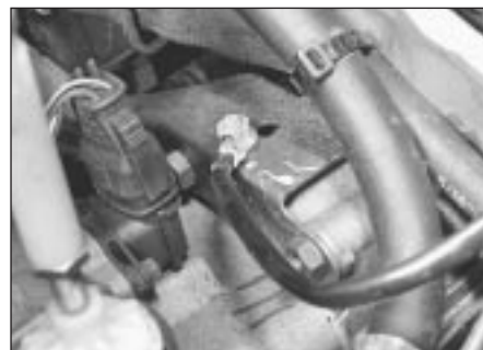
5.8c Earth strap to gearbox
