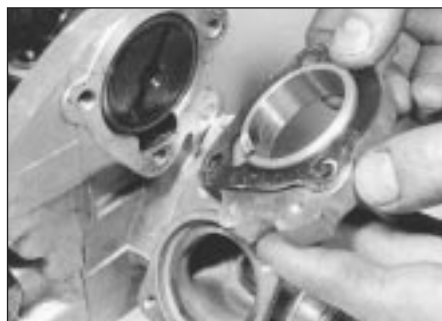
10.13 Removing distributor flange
