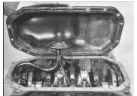
15.2 Removing the sump
