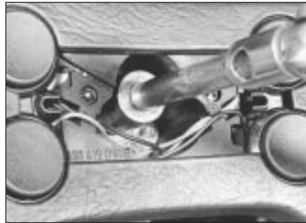
11.4 Undoing steering wheel retaining nut - GTi
