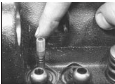
34.3 Locate plastic sleeve on valve stem . . .
