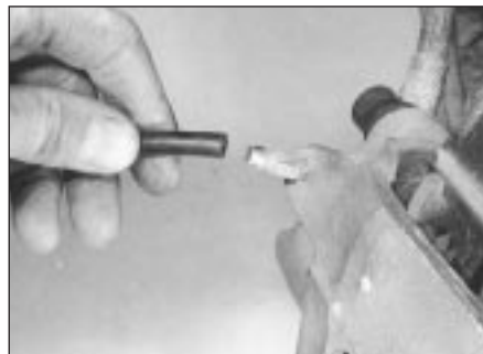
12.5 Connect bleed tube to bleed valve
