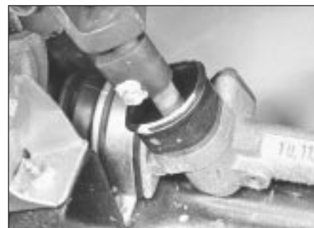
17.6 Steering gear pinion-to-lower column joint
