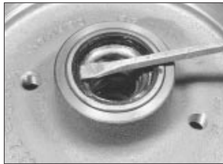
8.3 Prising out brake drum oil seal
