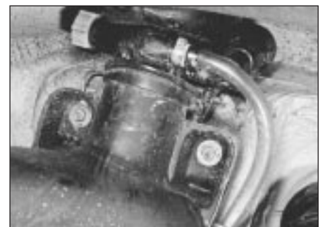
7.6 Fuel filler breather valve and hose
