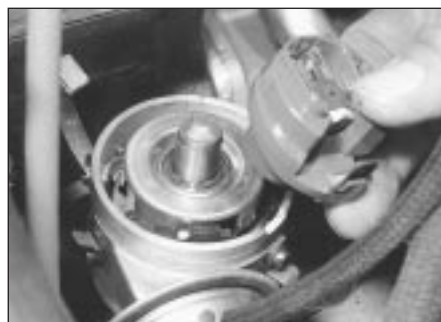
7.3a Pull free the rotor ...
