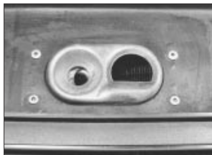
7.1 Bonnet lock and securing rivets
