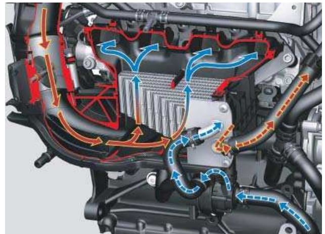
Dual-circuit cooling system with separate engine cooling and charge-air cooling circuits and plastic intake manifold with integrated charge air cooler
