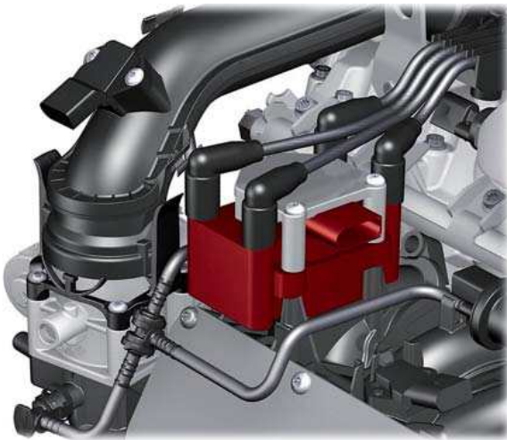
One ignition transformer for all four cylinders
