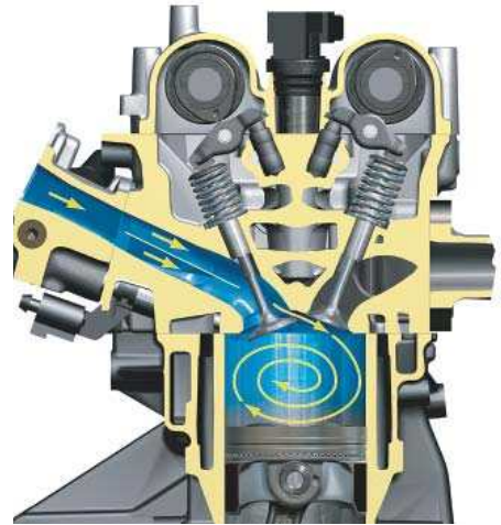
Four-valve cylinder head without intake manifold flaps
