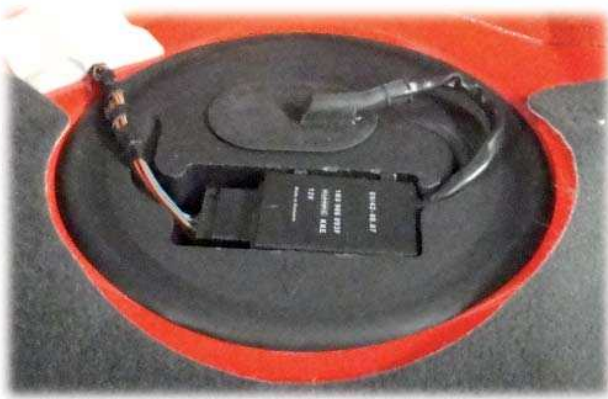
Demand-driven fuel system with fuel pump control unit
