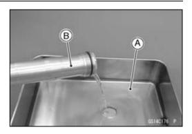
Clean the threads [A] of cylinder unit and base valve assembly.
