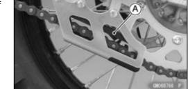
• Visually inspect the upper and lower chain guide rollers [A] and replace them if excessively worn or damaged.
