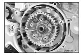
Remove: Toothed Washer [A] Clutch Housing [B]
