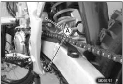
• Visually inspect the chain slipper [A] on the swingarm and replace it if excessively worn or damaged.
