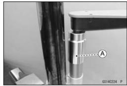
Inject the air of specified pressure to the balance chamber by using a suitable air pump [A].
