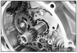
Install: Clutch Housing [A] Toothed Washer [B]
