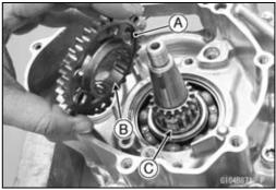
• Replace the circlip [A] with a new one, and install it to the output shaft.
