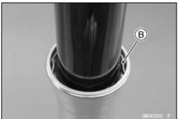
• Grasp the outer tube and stroke [A] the inner tube several times. The shock to fork seal separates the inner tube from the outer tube.
