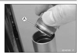
Tighten the plug bolt [A] to the specified torque.
