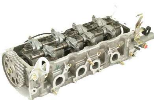
(Culata: vista exterior motor)
