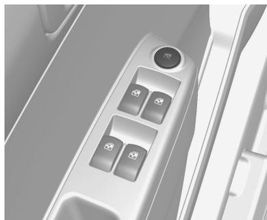
Pulse el interruptor
