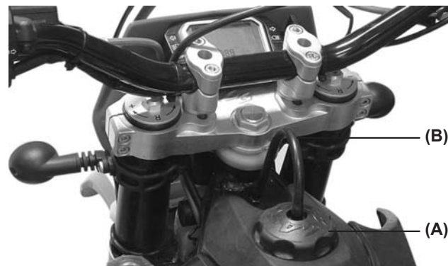
(A). Fuel cap. (B). Fuel vent hose.
