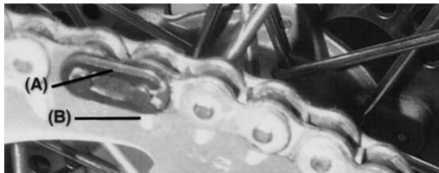
(A). Clip. (B). Chain direction of rotation.
