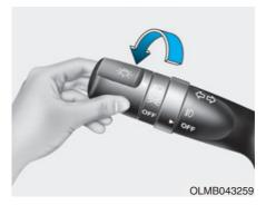
When the light switch is in the headlight position the head, tail, position, license and instrument panel lights are ON.
