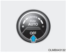
Press the front blower OFF button to turn off the front air climate control system. However, you can still operate the mode and air intake buttons as long as the ignition switch is in the ON position.
