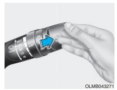
Push the lever away from you to spray rear washer fluid and to run the rear wipers 1~3 cycles. The spray and wiper operation will continue until you release the lever. (if equipped)
