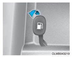
The fuel-filler lid must be opened from inside the vehicle by pulling up on the fuel-filler lid opener.
