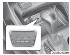
If your vehicle has an aux and/or USB (universal serial bus) port, you can use an aux port to connect audio devices and an USB port to plug in an USB and iPod<sup>®</sup>.
