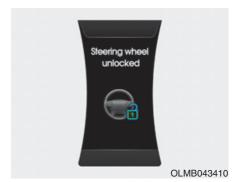
This warning message illuminates if the steering wheel does not lock when the Engine Start/Stop Button changes to the OFF position.
