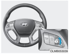
Push the lever (1) up (to RES+). If the vehicle speed is over 40 km/h (25 mph), the vehicle will resume the preset speed.
