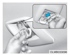
3. Insert the metal tab into the hole of the belt assembly cover.
