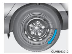
13. Use the wheel lug nut wrench to tighten the lug nuts in the order shown. Double-check each lug nut until they are tight. After changing tires, we recommend that an authorized HYUNDAI dealer tighten the lug nuts to their proper torque as soon as possible. The wheel lug nut should be tightened to 9~11 kg.m (65~79 lb.ft).
