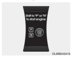
This warning message illuminates if you try to start the engine with the shift lever not in the P (Park) or N (Neutral) position.
