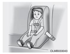
Installing a child restraint with a lap belt
