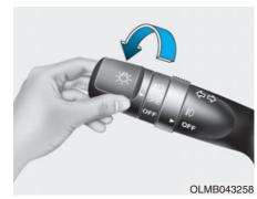
When the light switch is in the parking light position, the tail, position, license and instrument panel lights are ON.
