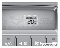
The current outside temperature is displayed in 1°C (1°F) increments. The temperature range is between -40°C  $\sim 60$ °C (-40°F  $\sim 140$ °F).
