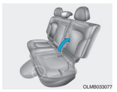
To use the rear seat, lift and push up the seatback backward. Push the seatback firmly until it clicks into place. Make sure the seatback is locked in place.
