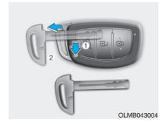
If the smart key does not operate normally, you can lock or unlock the doors by using the mechanical key.
