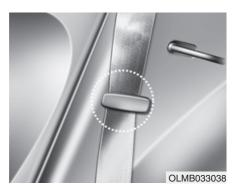
Routing the seat belt webbing through the rear seat belt guides will prevent the belts from being trapped behind or under the seats when the rear seats are folded down.
