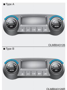
The temperature will increase to the maximum (HI) by turning the knob to the right extremely.
