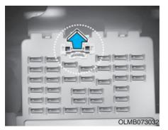
Your vehicle is equipped with a memory fuse (SHUNT connector) to prevent battery discharge if your vehicle is parked without being operated for prolonged periods. Use the following procedures before parking the vehicle for prolonged periods.
