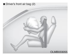
Upon deployment, tear seams molded directly into the pad covers will separate under pressure from the expansion of the air bags. Further opening of the covers allows full inflation of the air bags.
