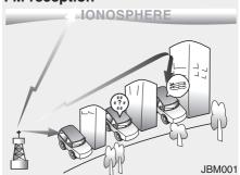
AM and FM radio signals are broadcast from transmitter towers located around your city. They are intercepted by the radio antenna on your vehicle. This signal is then received by the radio and sent to your vehicle speakers.
