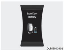
This warning message illuminates if the battery of the smart key is discharged when the Engine Start/Stop Button changes to the OFF position.
