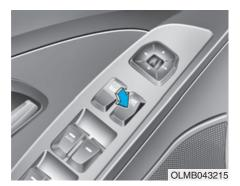
The driver can disable the power window switches on the front and rear passengers' doors by pressing the power window lock switch to lock position (pressed).
