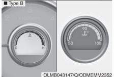
This gauge indicates the temperature of the engine coolant when the ignition switch or Engine Start/Stop button is ON
