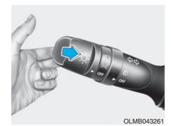
Pull the lever towards you. It will return to the normal position when released. The headlight switch does not need to be on to use this flashing feature.
