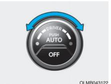
2. Set the Driver's temperature control switch to the desired temperature.
