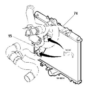
15 - air/water heat exchanger (inlet air heater)
