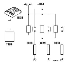
Assembly with 3 relays and 3 resistors
