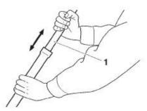
10.Antes measure the level of fork oil, wait ten minutes until the oil has settled and the air bubbles has dispersed.
