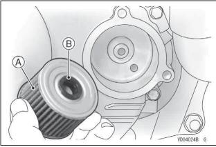
A. Oil Filter Element B. Grommet
