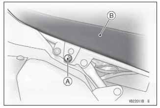
A. Bolt B. Seat • Disconnect the cables from the battery, first from the (-) terminal and then the (+) terminal.
