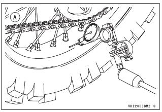
A. Radial Rim Runout Measurement
