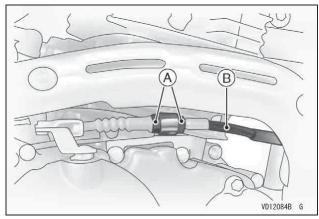
A. Locknuts B. Clutch Cable
