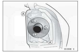
A. Spark Arrester Mounting Bolts
