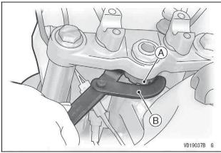
A. Steering Stem Locknut B. Stem Nut Wrench (P.N. 57001-1100)
