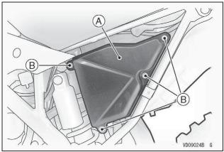
A. Air Cleaner Cover B. Bolts • Remove the wing bolt, and take out the air cleaner element.
