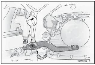
Apply an aerosol cable lubricant with a pressure lubricator on all cables:
