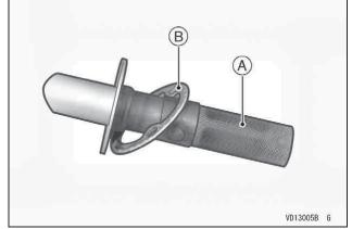
A. Spark Arrester B. Gasket
