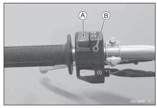
A. Engine Stop Switch B. Indicator Light (LED)
