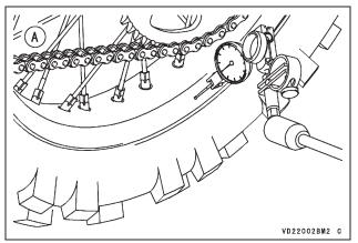
A. Axial Rim Runout Measurement
