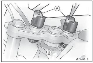
A. Handlebar Holders B. Handlebar Holder Nuts
