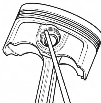
Removing the Gudgeon Pin Circlip
