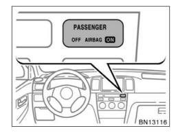
The front passenger occupant classification indicator light indicates the actuation of the front passenger airbag, side airbag on the front passenger seat and front passenger's seat belt pretensioner.
