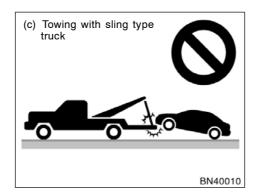
(c) Towing with sling type truck
