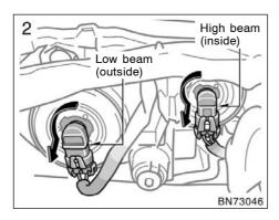
2. Turn the bulb base counterclockwise to the front of the vehicle as shown.
