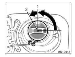
2. To remove the fuel tank cap, turn the cap counterclockwise by 90 degrees (to the pressure point 1), and then turn it an additional 30 degrees (to point 2). Pause slightly before removing it.
