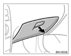
To open the glove box door, pull the lever.
