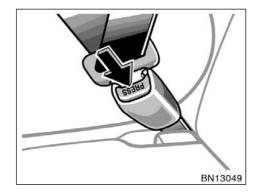
4. To remove the infant seat, press the buckle release button and allow the belt to retract completely. The belt will move freely again and be ready to work for an adult or older child passenger.
