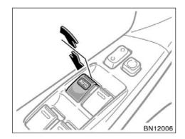
The windows can be operated with the switch on each door.
