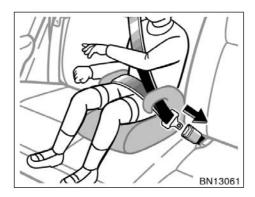
Sit the child on a booster seat. Run the lap and shoulder belt through or around the booster seat and across the child following the instructions provided by its manufacturer and insert the tab into the buckle taking care not to twist the belt.
