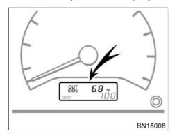
The outside temperature is indicated on the display when the ignition switch is on.
