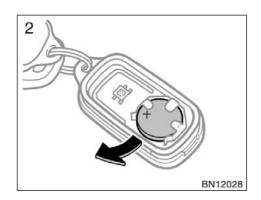
2. Remove the discharged transmitter battery.
