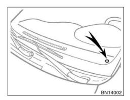
The daytime running light control sensor is on the top of the driver's side instrument panel.
