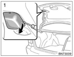
Use a flat-bladed screwdriver or equivalent.
