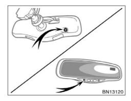
To ensure correct functioning of an anti-glare mirror sensors located on the back side of the mirror, do not touch or cover the sensors with your finger or a piece of cloth, etc.
