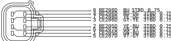
5W7T-14A464-6A(XXX) C11CA TO 12A690 9F666 INLINE HARNESS 12A690
