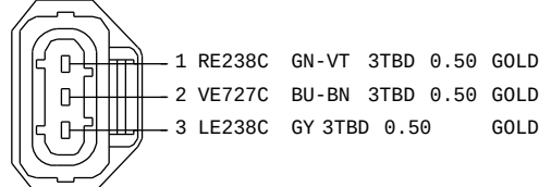
1L2T-14A464-UA C1E727C TO FUEL RAIL PRESSURE SENSOR HARNESS 12A690
